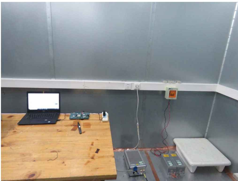
Picture 2 Conducted Emission Test Setup
