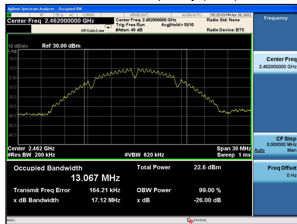
802.11b, Carrier frequency (MHz): 2462
