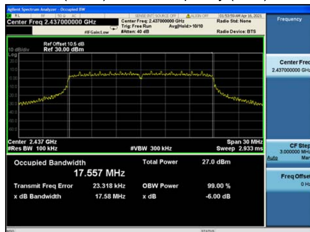
802.11n(HT20), Carrier frequency (MHz): 2462
