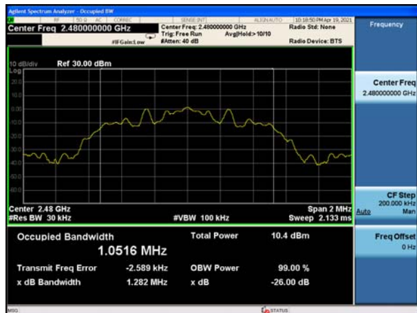
Bluetooth LE (125K) Carrier frequency (MHz): 2480
