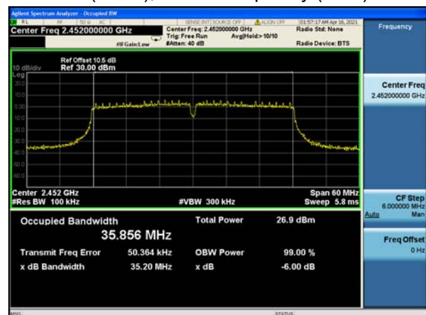
802.11n(HT40), Carrier frequency (MHz): 2452
