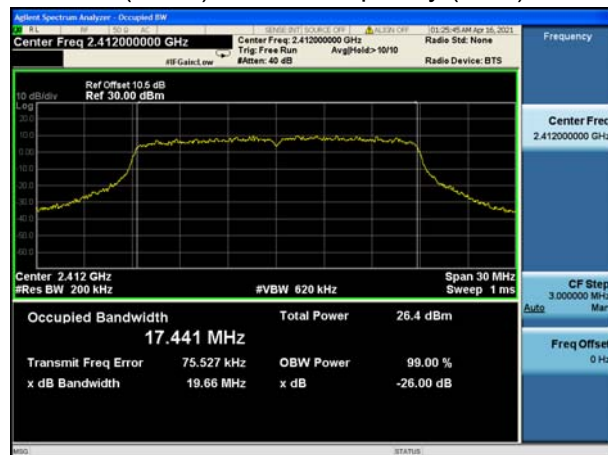
802.11n(HT20), Carrier frequency (MHz): 2437
