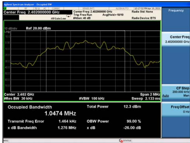
Bluetooth LE (125K) Carrier frequency (MHz): 2440
