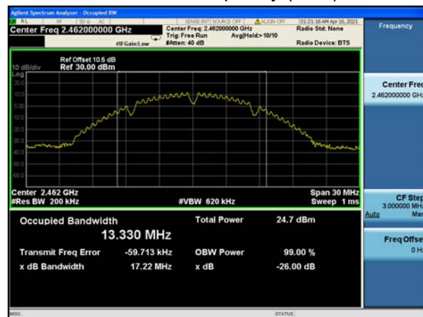
802.11b, Carrier frequency (MHz): 2462
