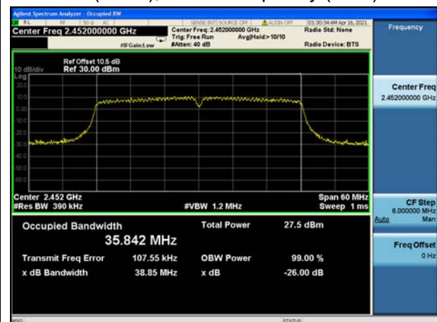
802.11n(HT40), Carrier frequency (MHz): 2452
