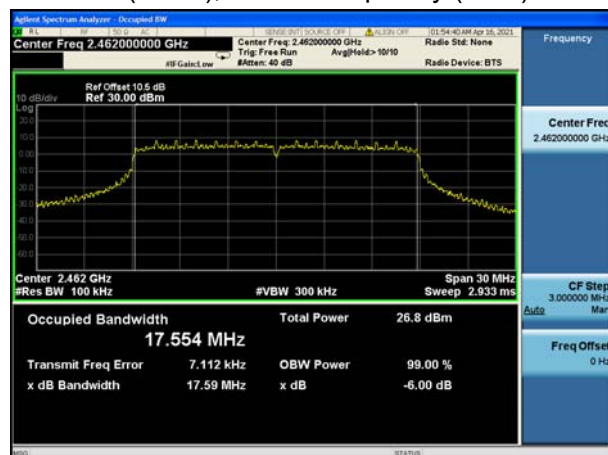
802.11n(HT20), Carrier frequency (MHz): 2462
