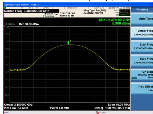
BT DH5 CH78, Carrier frequency (MHz): 2480
