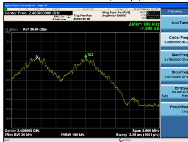
BT DH5 CH78, Carrier frequency (MHz): 2480
