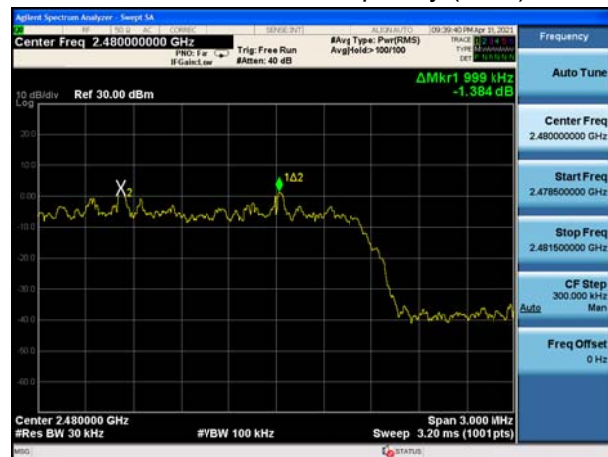
BT 2DH5 CH78, Carrier frequency (MHz): 2480
