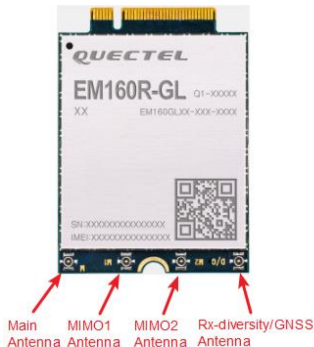
Figure 32: Antenna Connectors on the EM160R-GL Module
