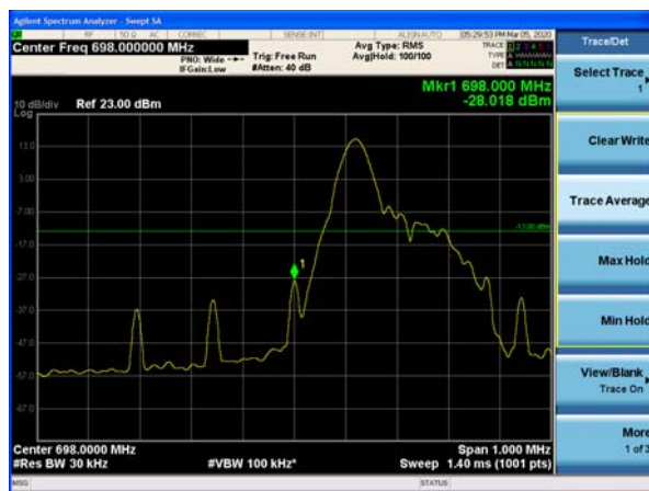
NB-IOT Band 85 QPSK 15kHz 12@0 CH-Low
