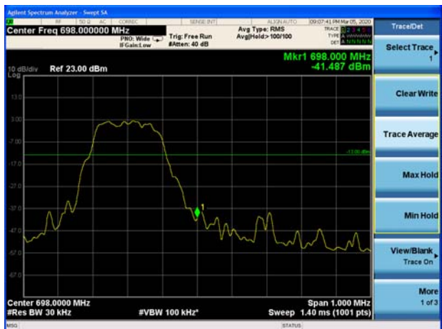
NB-IOT Band 71 QPSK 15kHz 12@0 CH-High
