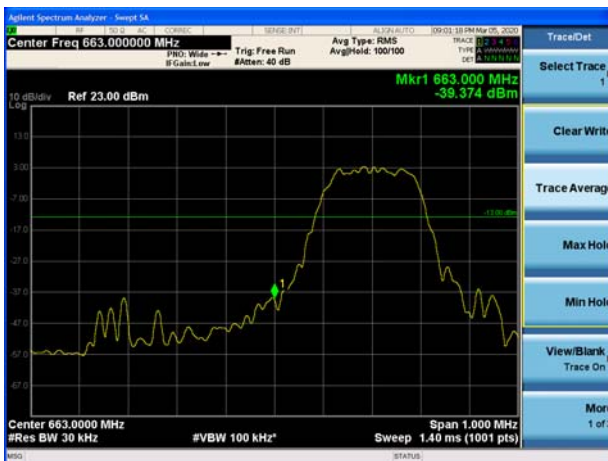
NB-IOT Band 71 QPSK 15kHz 12@0 CH-Low
