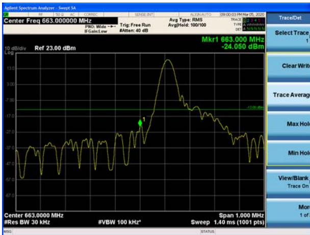
NB-IOT Band 71 QPSK 15kHz 1@0 CH-Low
