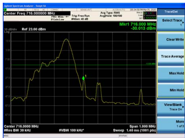
NB-IOT Band 85 QPSK 15kHz 12@0 CH-High
