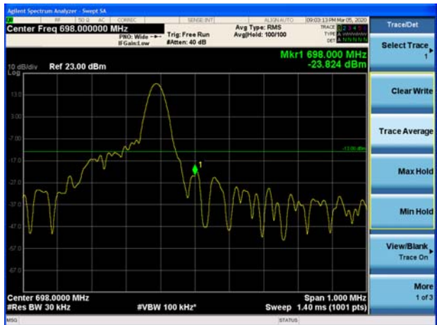
NB-IOT Band 71 QPSK 15kHz 1@11 CH-High
