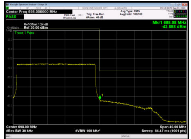
LTE Band 71 64QAM 5MHz CH-High, 1 RB
