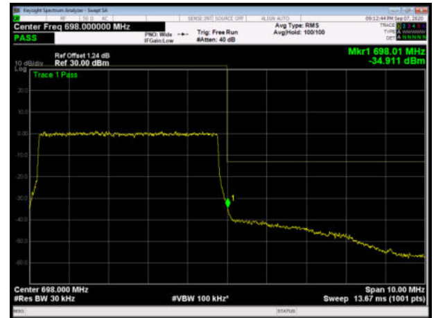
LTE Band 71 64QAM 5MHz CH-High, 100%RB
