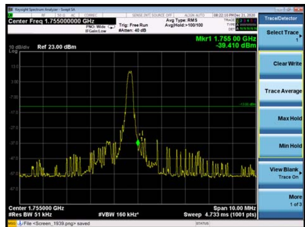
LTE Band 4 QPSK 5MHz CH-High, 100%RB
