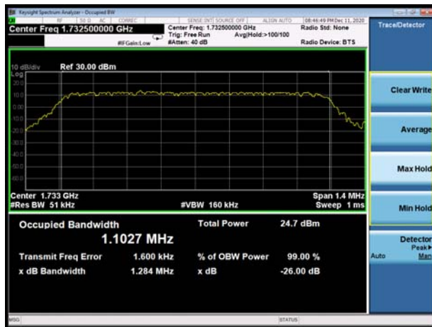
LTE Band 4 QPSK 5MHz CH-Middle
