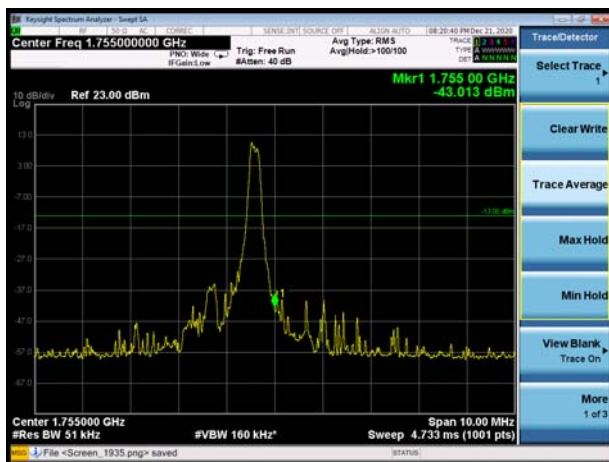
LTE Band 4 QPSK 3MHz CH-High, 1 RB
