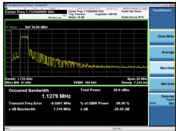
LTE Band 4 QPSK 20MHz CH-Middle
