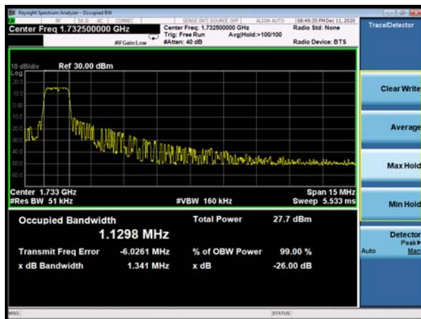
LTE Band 4 QPSK 15MHz CH-Middle
