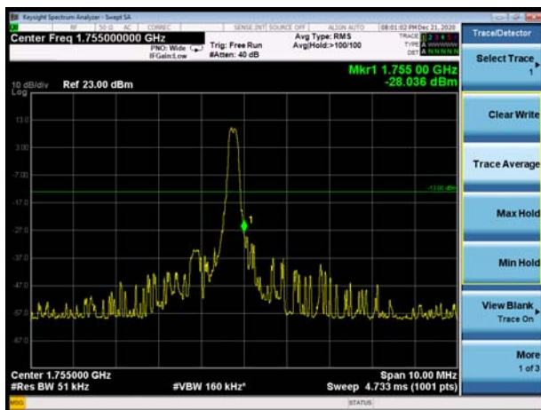
LTE Band 4 QPSK 1.4MHz CH-High, 100%RB
