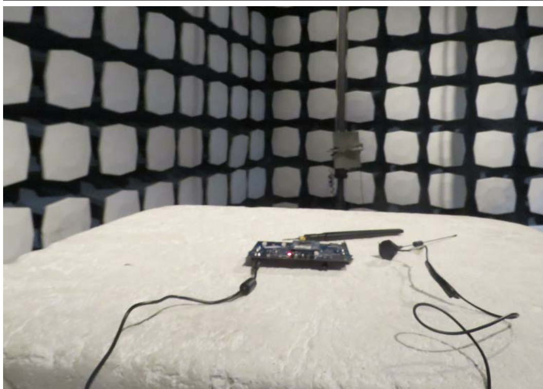
Picture 1: Radiated Spurious Emissions Test setup
