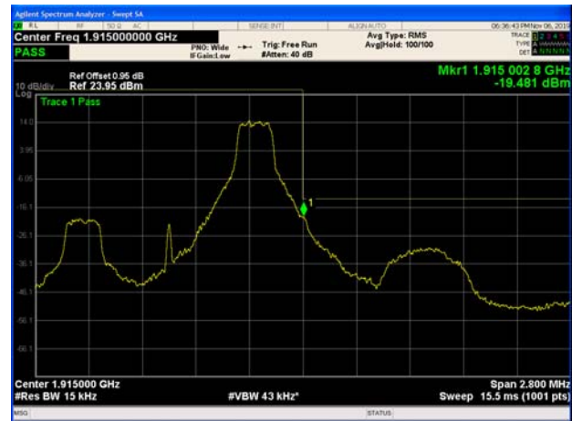
LTE Band 25 1.4MHz QPSK 100%RB CH-High
