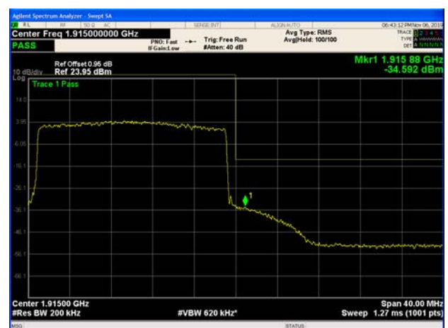
LTE Band 25 20MHz 16QAM 100%RB CH-High
