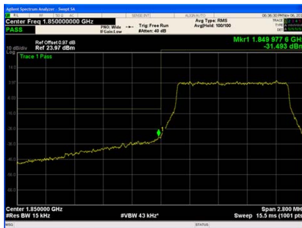
LTE Band 25 3MHz 16QAM 1RB CH-Low
