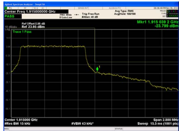
LTE Band 25 3MHz QPSK 1RB CH-High
