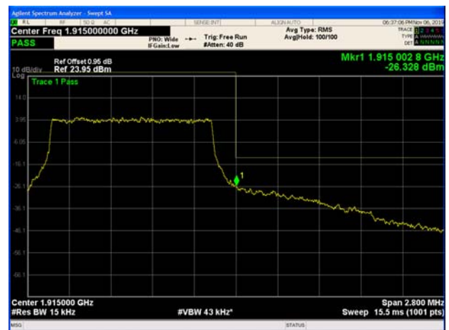
LTE Band 25 3MHz 16QAM 1RB CH-High
