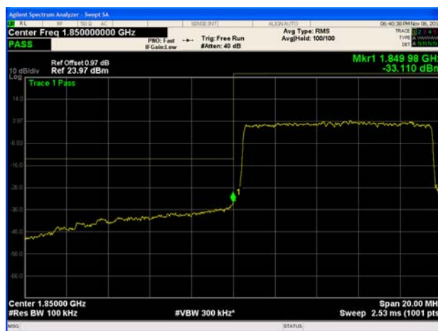
LTE Band 25 15MHz 16QAM 1RB CH-Low
