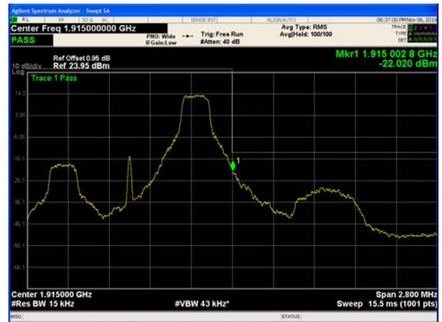
LTE Band 25 1.4MHz 16QAM 100%RB CH-High
