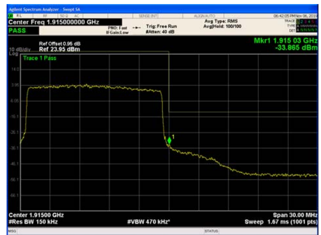
LTE Band 25 20MHz 16QAM 1RB CH-High
