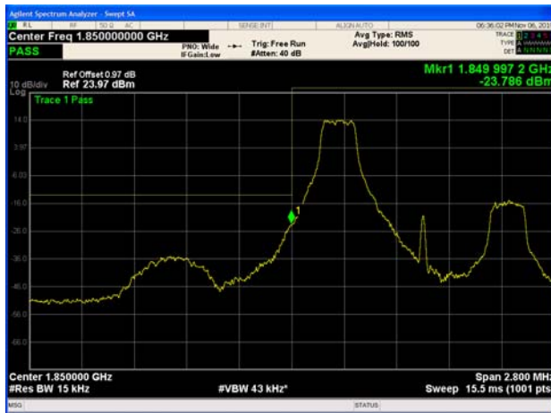
LTE Band 25 1.4MHz QPSK 100%RB CH-Low
