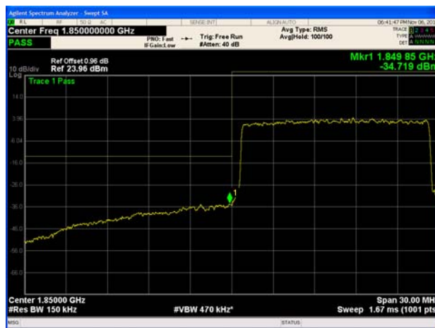
LTE Band 25 20MHz 16QAM 1RB CH-Low
