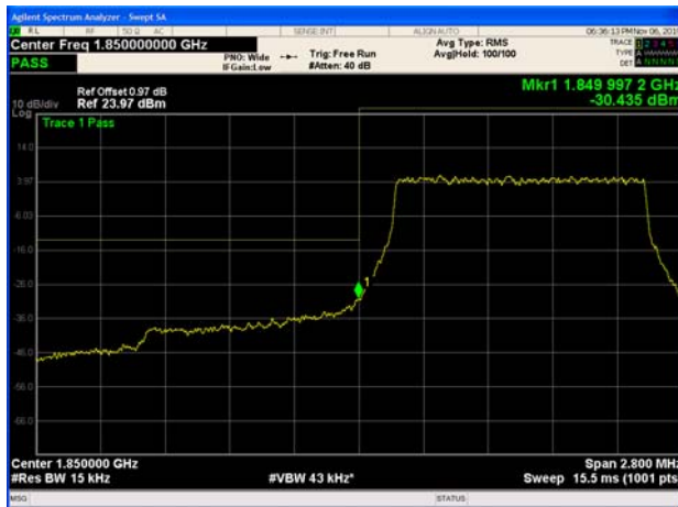
LTE Band 25 3MHz QPSK 1RB CH-Low
