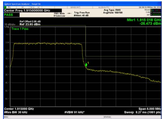
LTE Band 25 5MHz 16QAM 1RB CH-High
