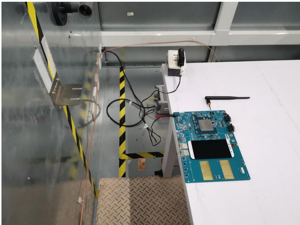
**Radiated Emissions Test Photos****30 MHz to 1000 MHz**
