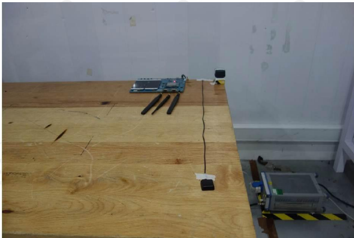
Power Line Conducted Emissions
