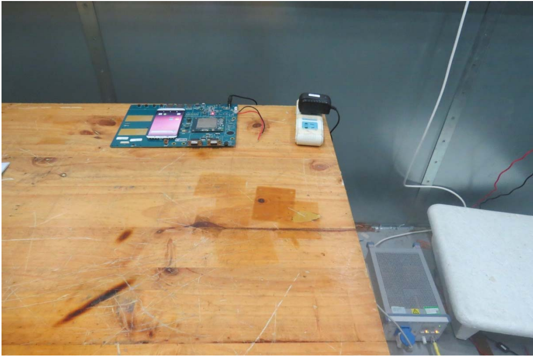
Picture 2 Conducted Emission Test Setup
