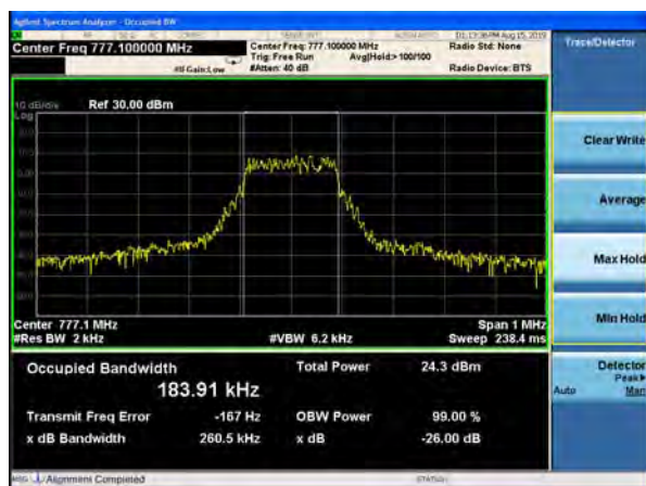
NB-IOT Band 13 QPSK 15kHz 12@0 CH-Middle
