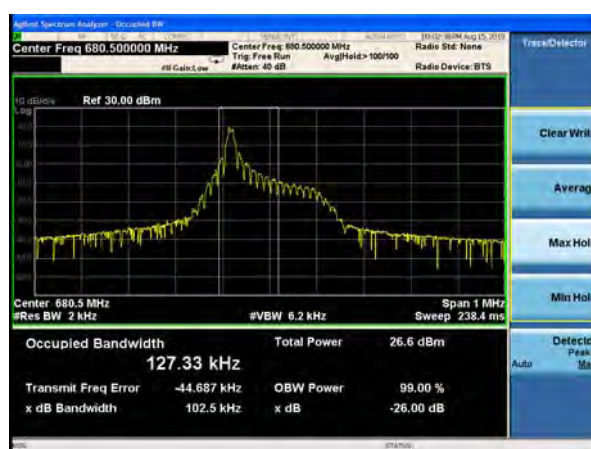
NB-IOT Band 71 BPSK 15kHz 1@0 CH-High
