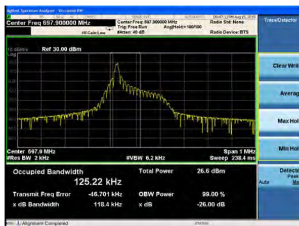
NB-IOT Band 71 BPSK 15kHz 1@0 CH-High
