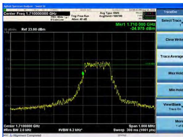
NB-IOT Band 4 QPSK 15kHz 12@0 CH-Low
