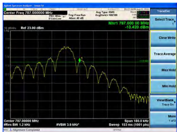
NB-IOT Band 13 QPSK 15kHz 12@0 CH-High
