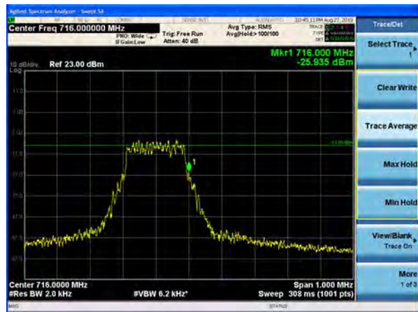
NB-IOT Band 85 QPSK 15kHz 12@0 CH-High
