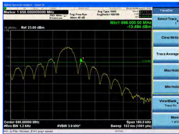
NB-IOT Band 71 QPSK 15kHz 12@0 CH-High
