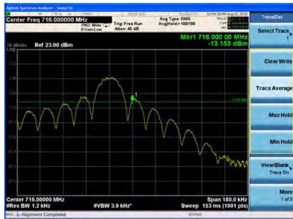
NB-IOT Band 85 QPSK 15kHz 12@0 CH-High
