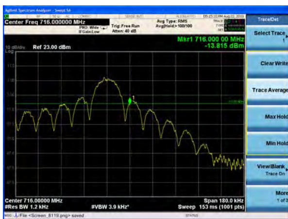
NB-IOT Band 12 QPSK 15kHz 12@0 CH-High
