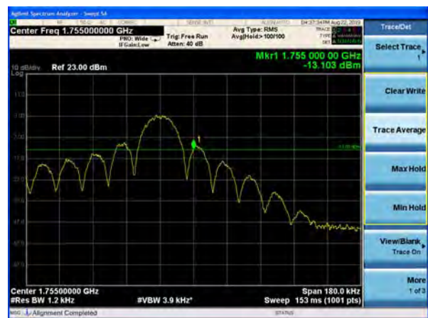
NB-IOT Band 4 QPSK 15kHz 12@0 CH-High
