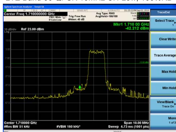
LTE Band 66 QPSK 15MHz CH-Low, 1 RB
