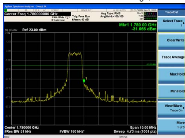
LTE Band 66 16QAM 3MHz CH-High, 1 RB
