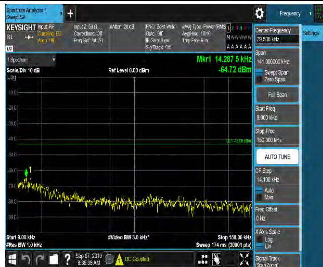
LTE Band 2_20MHz_QPSK_18900_1RB#0_Range2:0.15~30MHz_-60.33_PASS
