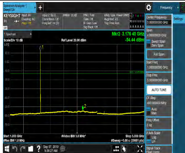
LTE Band 2_5MHz_16QAM_19175_1RB#0_Range5:5000~12000MHz_-64.94_PASS
