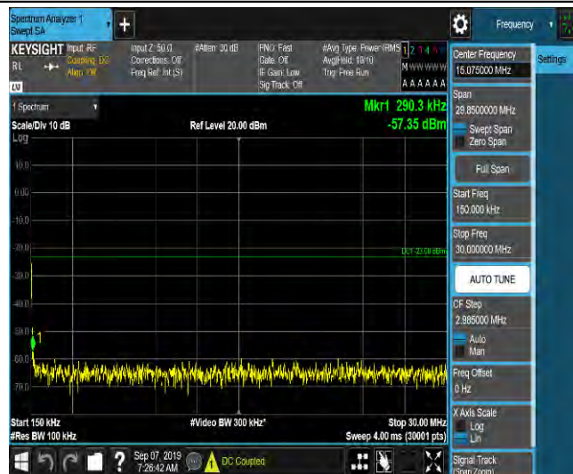
LTE Band 2_20MHz_16QAM_18700_1RB#0_Range3:30~1000MHz_-47.66_PASS
