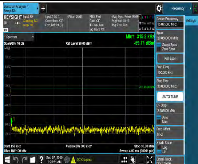
LTE Band 2_10MHz_16QAM_19150_1RB#0_Range3:30~1000MHz_-47_PASS
