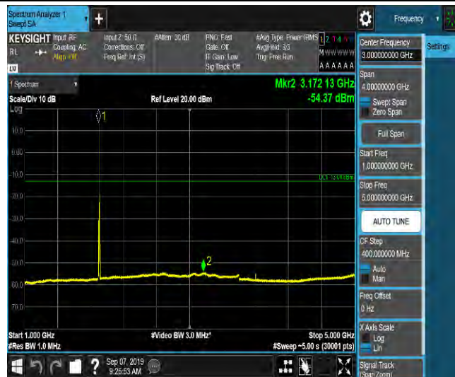
LTE Band 2_10MHz_QPSK_19150_1RB#0_Range5:5000~12000MHz_-64.39_PASS
