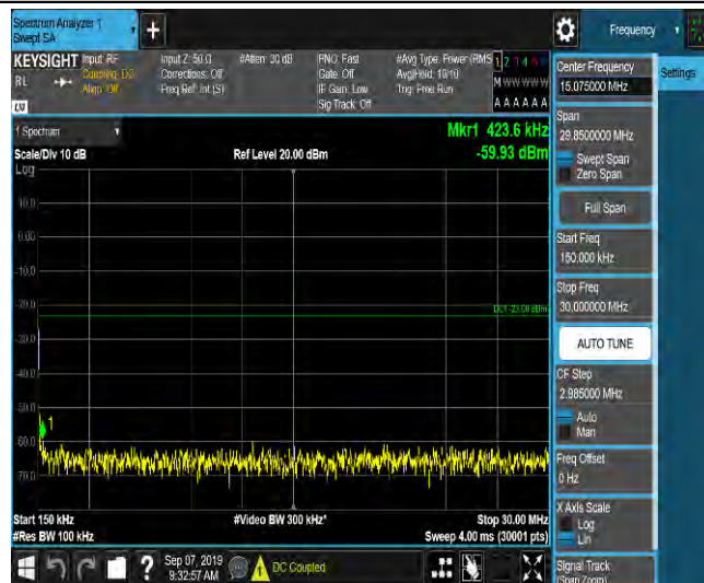
LTE Band 2_5MHz_16QAM_18900_1RB#0_Range3:30~1000MHz_-47.63_PASS
