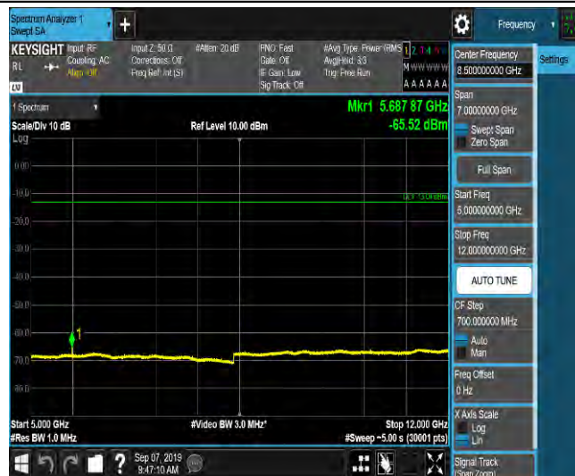
LTE Band 2_15MHz_16QAM_19125_1RB#0_Range6:12000~18000MHz_-55.45_PASS
