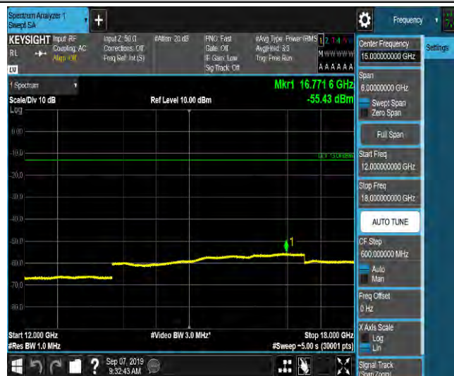
LTE Band 2_5MHz_16QAM_18900_1RB#0_Range1:0.009~0.15MHz_-63.77_PASS
