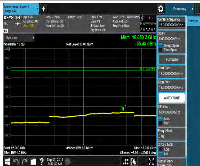
LTE Band 2_20MHz_QPSK_18700_1RB#0_Range1:0.009~0.15MHz_-62.03_PASS
