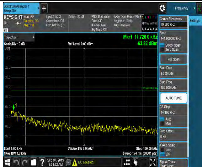
LTE Band 2_5MHz_QPSK_18900_1RB#0_Range2:0.15~30MHz_-59.72_PASS
