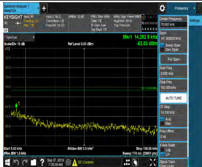
LTE Band 2_20MHz_QPSK_18700_1RB#0_Range2:0.15~30MHz_-56.08_PASS
