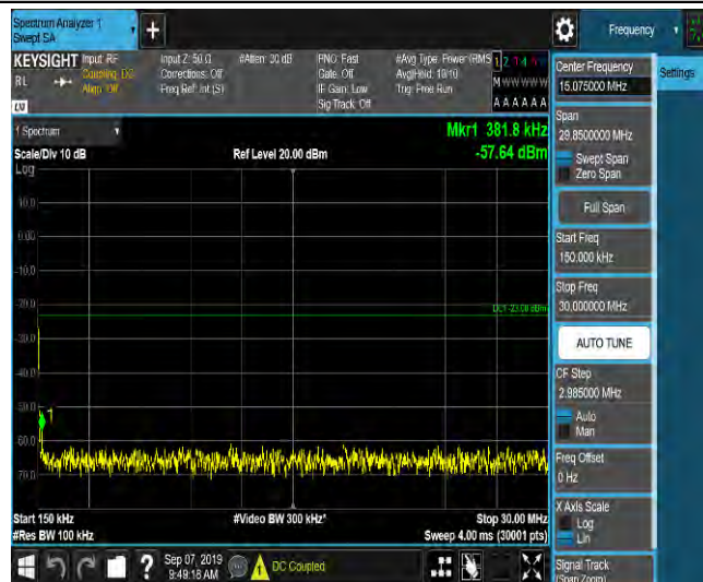
LTE Band 2_3MHz_16QAM_18900_1RB#0_Range3:30~1000MHz_-46.69_PASS
