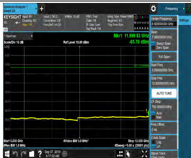
LTE Band 2_10MHz_QPSK_18650_1RB#0_Range6:12000~18000MHz_-55.37_PASS
