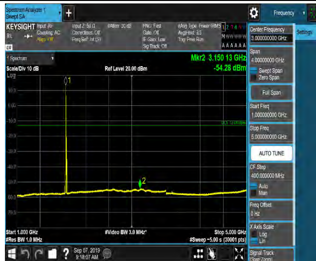
LTE Band 2_10MHz_16QAM_18650_1RB#0_Range5:5000~12000MHz_-65.69_PASS
