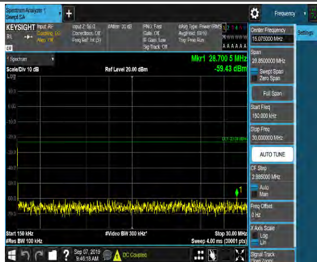
LTE Band 2_15MHz_16QAM_19125_1RB#0_Range3:30~1000MHz_-45.92_PASS
