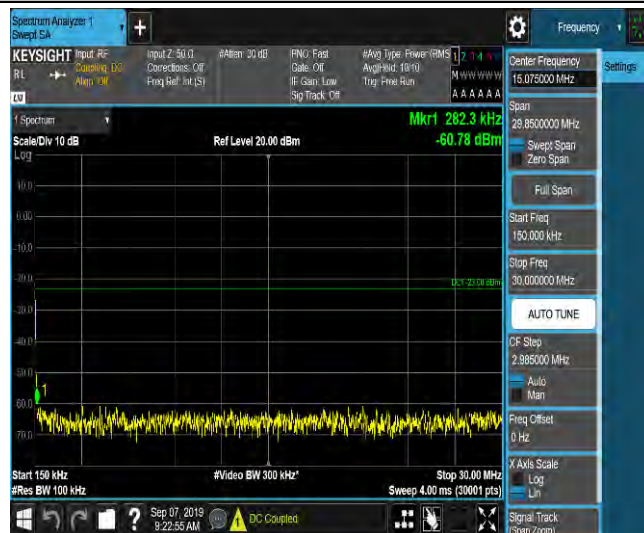
LTE Band 2_10MHz_16QAM_18900_1RB#0_Range3:30~1000MHz_-46.56_PASS
