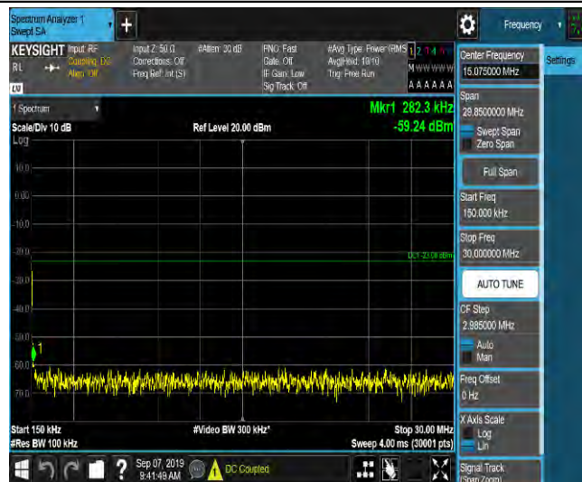
LTE Band 2_15MHz_QPSK_18900_1RB#0_Range3:30~1000MHz_-48.27_PASS
