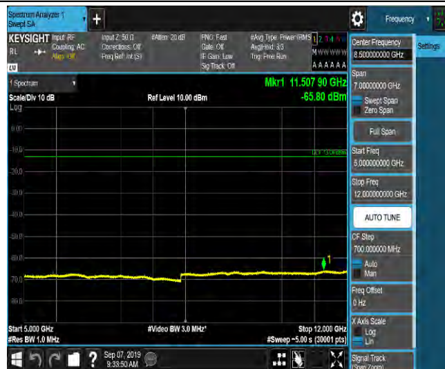
LTE Band 2_5MHz_16QAM_18900_1RB#0_Range6:12000~18000MHz_-55.48_PASS
