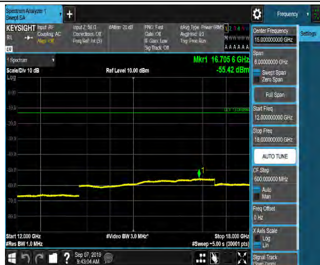
LTE Band 2_15MHz_16QAM_18900_1RB#0_Range1:0.009~0.15MHz_-63.64_PASS
