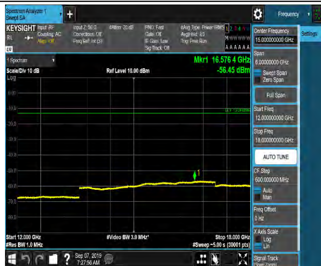
LTE Band 2_20MHz_QPSK_18900_1RB#0_Range1:0.009~0.15MHz_-64.72_PASS
