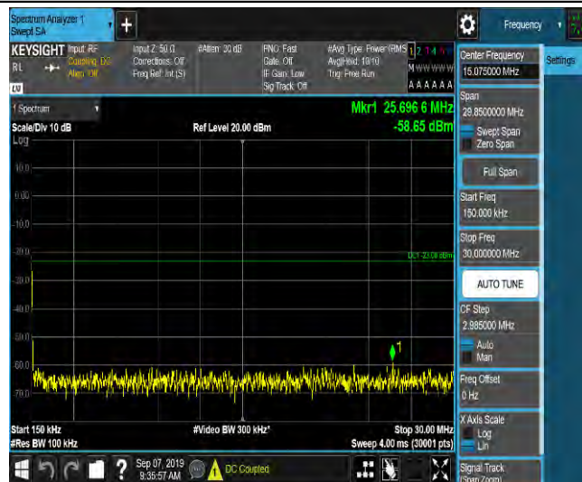
LTE Band 2_5MHz_16QAM_19175_1RB#0_Range3:30~1000MHz_-47.77_PASS
