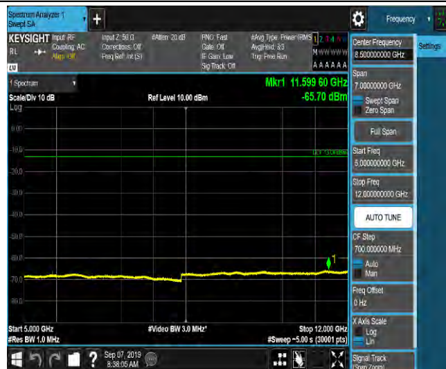
LTE Band 2_20MHz_16QAM_18900_1RB#0_Range6:12000~18000MHz_-55.36_PASS
