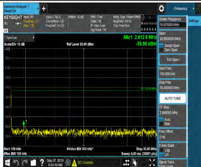
LTE Band 2_15MHz_QPSK_19125_1RB#0_Range3:30~1000MHz_-47.59_PASS
