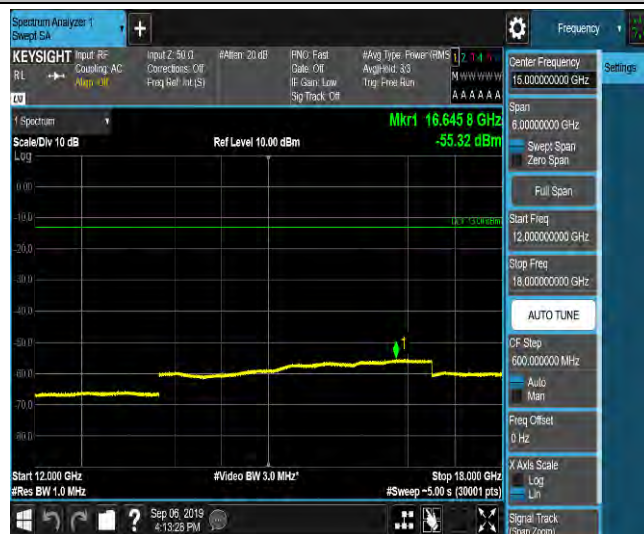
LTE Band 2_3MHz_QPSK_18900_1RB#0_Range1:0.009~0.15MHz_-63.48_PASS
