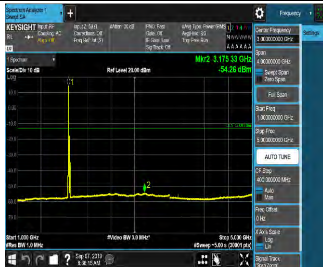
LTE Band 2_20MHz_QPSK_18900_1RB#0_Range5:5000~12000MHz_-65.76_PASS
