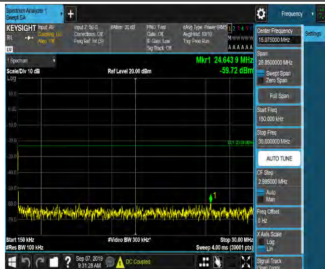
LTE Band 2_5MHz_QPSK_18900_1RB#0_Range3:30~1000MHz_-46.5_PASS
