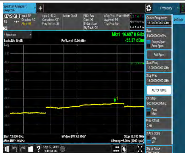
LTE Band 2_3MHz_16QAM_18900_1RB#0_Range1:0.009~0.15MHz_-63.32_PASS
