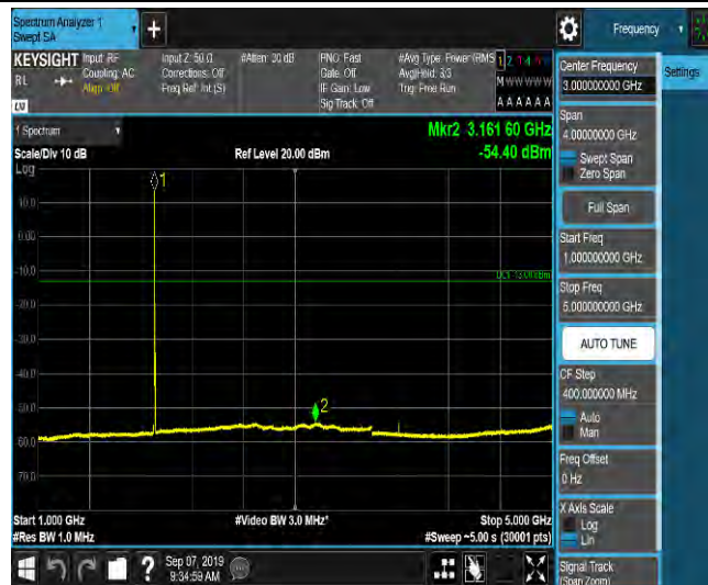
LTE Band 2_5MHz_QPSK_19175_1RB#0_Range5:5000~12000MHz_-63.86_PASS
