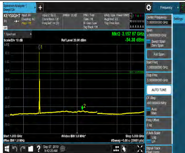
LTE Band 2_15MHz_QPSK_18900_1RB#0_Range5:5000~12000MHz_-65.7_PASS
