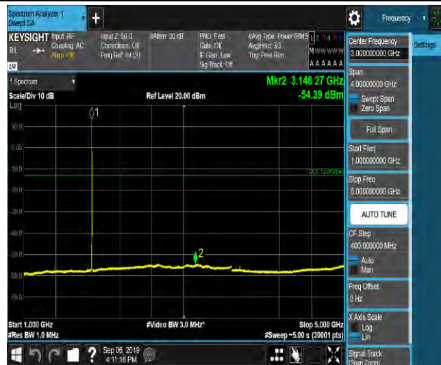
LTE Band 2_3MHz_QPSK_18615_1RB#0_Range5:5000~12000MHz_-65.64_PASS
