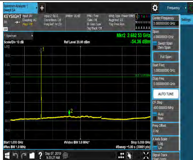
LTE Band 2_5MHz_16QAM_18900_1RB#0_Range5:5000~12000MHz_-65.8_PASS
