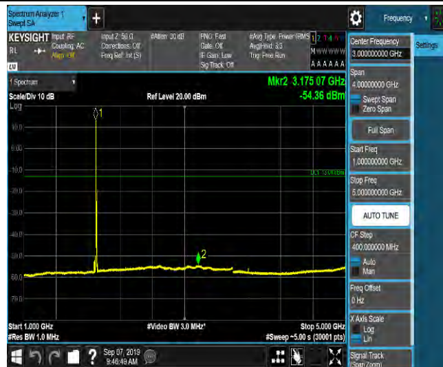
LTE Band 2_15MHz_16QAM_19125_1RB#0_Range5:5000~12000MHz_-65.52_PASS
