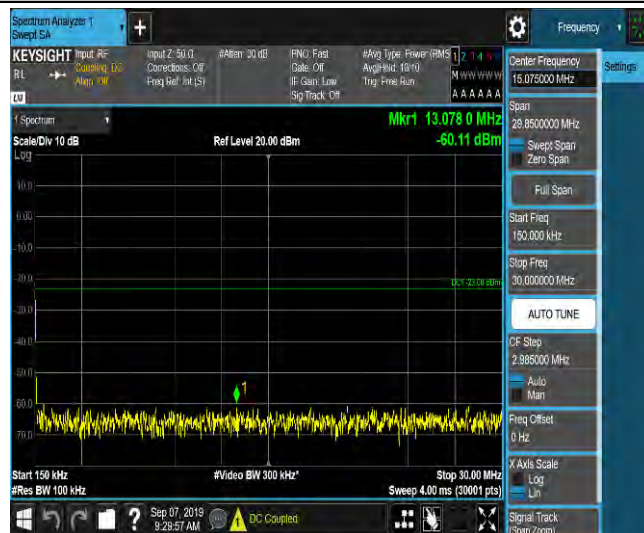
LTE Band 2_5MHz_16QAM_18625_1RB#0_Range3:30~1000MHz_-47.9_PASS
