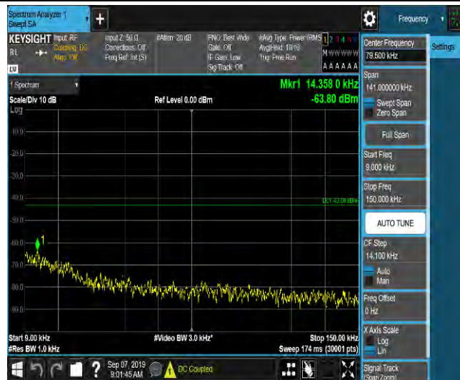
LTE Band 2_20MHz_16QAM_19100_1RB#0_Range2:0.15~30MHz_-59.09_PASS
