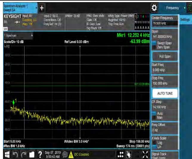
LTE Band 2_3MHz_QPSK_19185_1RB#0_Range2:0.15~30MHz_-60.14_PASS
