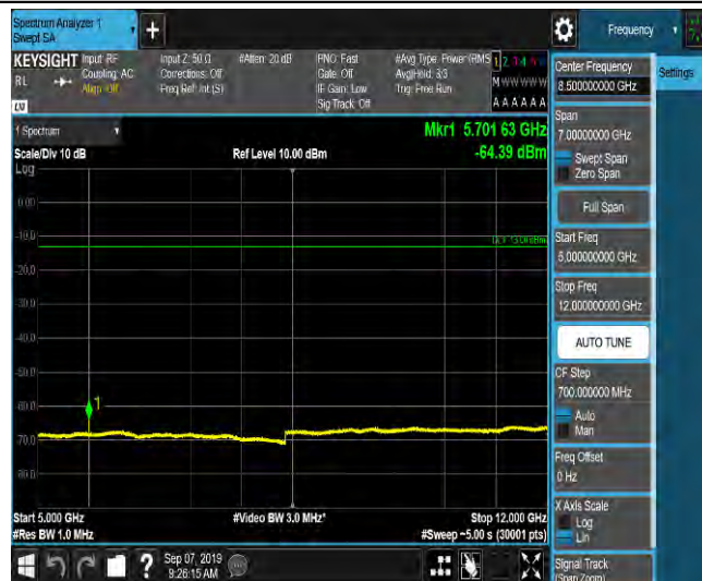
LTE Band 2_10MHz_QPSK_19150_1RB#0_Range6:12000~18000MHz_-55.42_PASS
