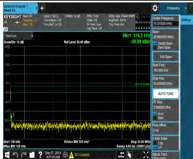
LTE Band 2_20MHz_16QAM_19100_1RB#0_Range3:30~1000MHz_-46.22_PASS
