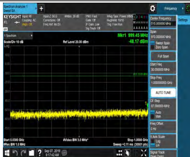
LTE Band 2_10MHz_16QAM_18650_1RB#0_Range4:1000~5000MHz_-54.28_PASS
