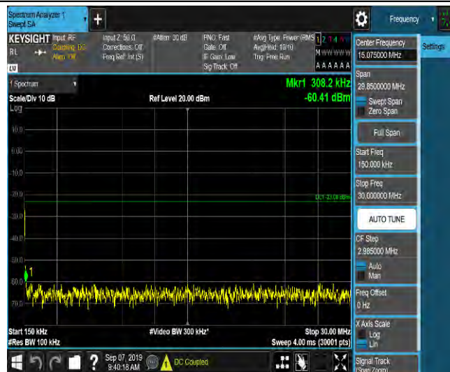
LTE Band 2_15MHz_16QAM_18675_1RB#0_Range3:30~1000MHz_-46.16_PASS
