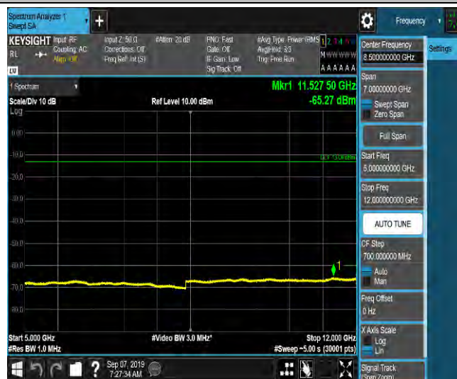
LTE Band 2_20MHz_16QAM_18700_1RB#0_Range6:12000~18000MHz_-56.45_PASS
