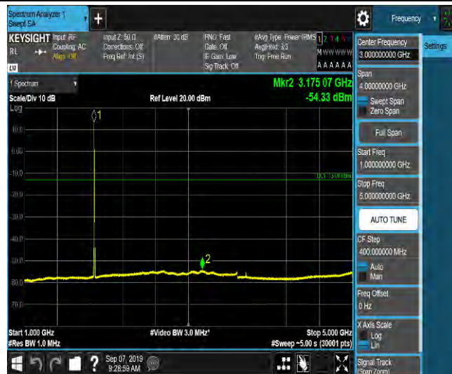
LTE Band 2_5MHz_QPSK_18625_1RB#0_Range5:5000~12000MHz_-65.85_PASS
