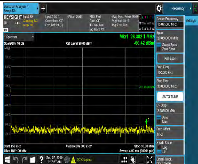
LTE Band 2_10MHz_16QAM_18650_1RB#0_Range3:30~1000MHz_-48.17_PASS
