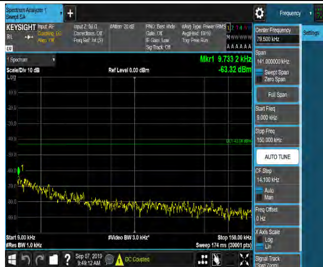
LTE Band 2_3MHz_16QAM_18900_1RB#0_Range2:0.15~30MHz_-57.64_PASS
