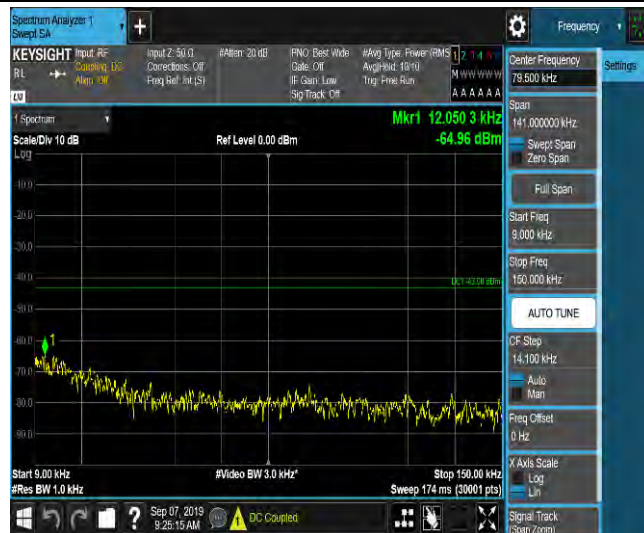
LTE Band 2_10MHz_QPSK_19150_1RB#0_Range2:0.15~30MHz_-59_PASS
