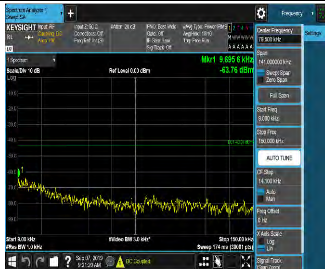
LTE Band 2_10MHz_QPSK_18900_1RB#0_Range2:0.15~30MHz_-58.89_PASS
