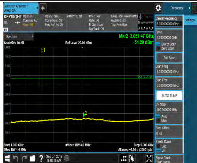
LTE Band 2_3MHz_QPSK_18900_1RB#0_Range5:5000~12000MHz_-65.43_PASS
