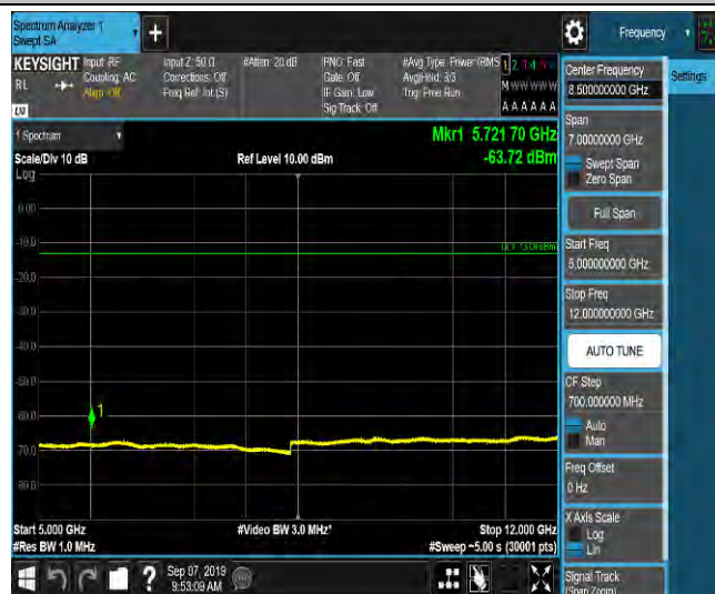
LTE Band 2_3MHz_16QAM_19185_1RB#0_Range6:12000~18000MHz_-55.47_PASS
