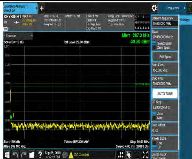
LTE Band 2_3MHz_16QAM_18615_1RB#0_Range3:30~1000MHz_-47.47_PASS
