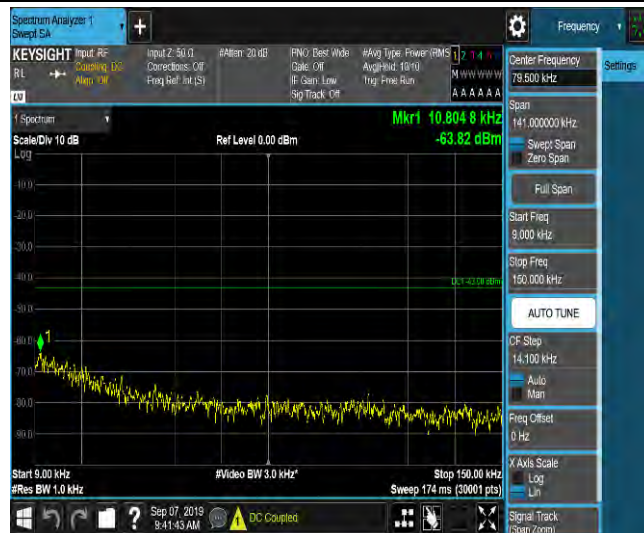
LTE Band 2_15MHz_QPSK_18900_1RB#0_Range2:0.15~30MHz_-59.24_PASS
