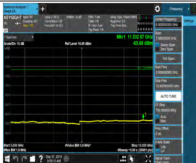
LTE Band 2_3MHz_16QAM_18900_1RB#0_Range6:12000~18000MHz_-55.31_PASS
