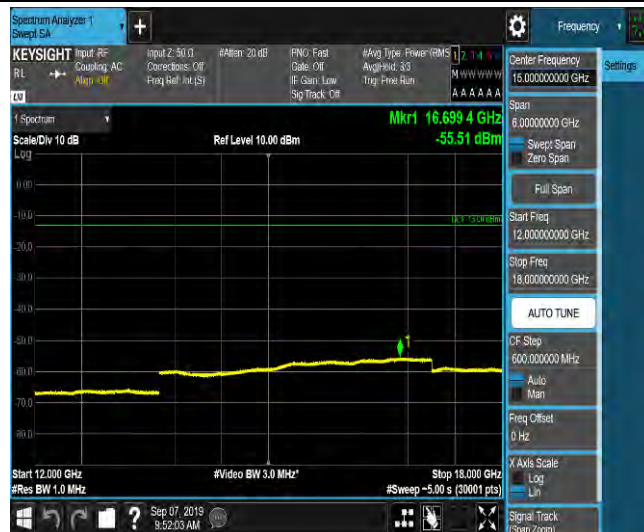
LTE Band 2_3MHz_16QAM_19185_1RB#0_Range1:0.009~0.15MHz_-64.32_PASS
