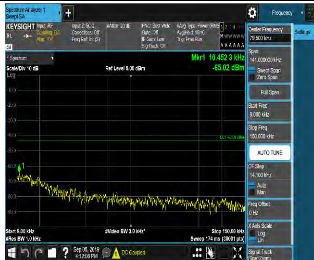
LTE Band 2_3MHz_16QAM_18615_1RB#0_Range2:0.15~30MHz_-59.5_PASS
