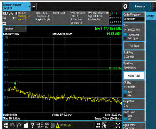
LTE Band 2_3MHz_16QAM_19185_1RB#0_Range2:0.15~30MHz_-60.05_PASS
