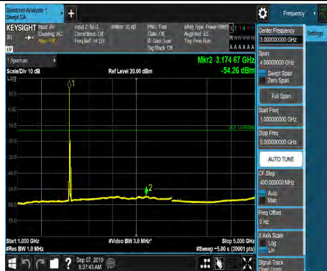
LTE Band 2_20MHz_16QAM_18900_1RB#0_Range5:5000~12000MHz_-65.7_PASS
