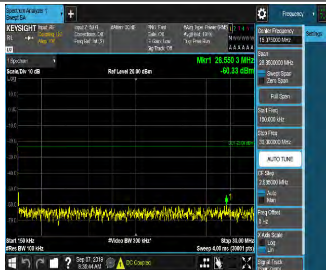
LTE Band 2_20MHz_QPSK_18900_1RB#0_Range3:30~1000MHz_-47.6_PASS
