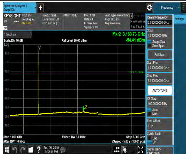
LTE Band 2_3MHz_16QAM_18615_1RB#0_Range5:5000~12000MHz_-65.7_PASS
