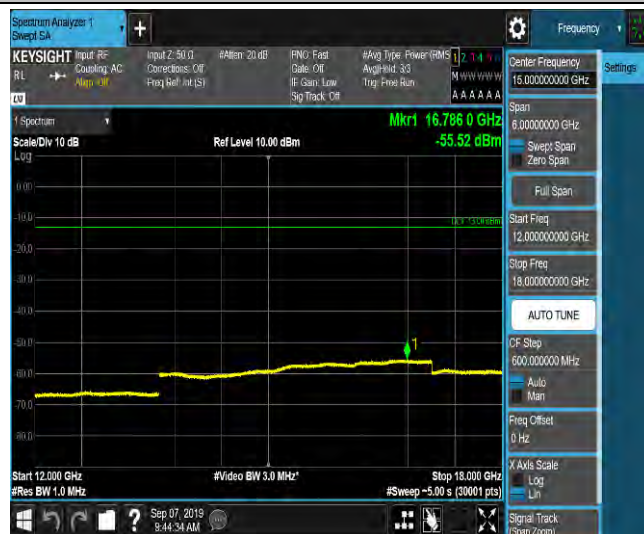
LTE Band 2_15MHz_QPSK_19125_1RB#0_Range1:0.009~0.15MHz_-63.8_PASS
