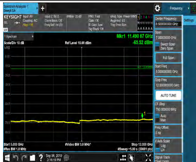
LTE Band 2_1.4MHz_QPSK_18607_1RB#0_Range6:12000~18000MHz_-55.35_PASS
