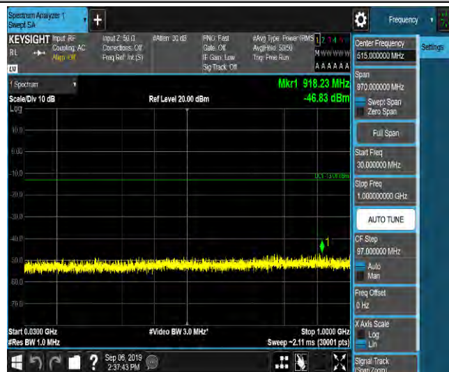
LTE Band 2_1.4MHz_QPSK_18900_1RB#0_Range4:1000~5000MHz_-54.5_PASS
