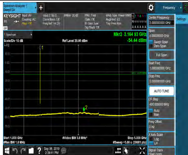
LTE Band 2_1.4MHz_16QAM_18900_1RB#0_Range5:5000~12000MHz_-65.13_PASS
