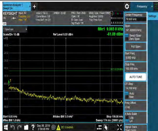
LTE Band 2_1.4MHz_16QAM_18900_1RB#0_Range2:0.15~30MHz_-59.29_PASS
