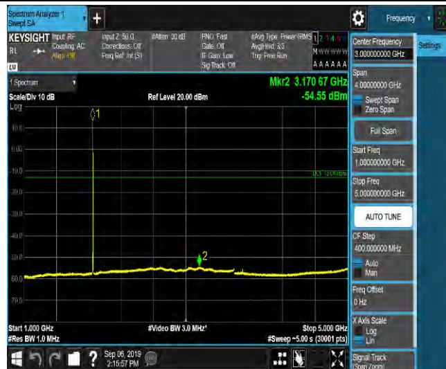
LTE Band 2_1.4MHz_QPSK_18607_1RB#0_Range5:5000~12000MHz_-65.52_PASS
