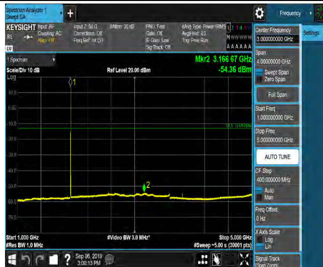
LTE Band 2_1.4MHz_QPSK_19193_1RB#0_Range5:5000~12000MHz_-63.23_PASS
