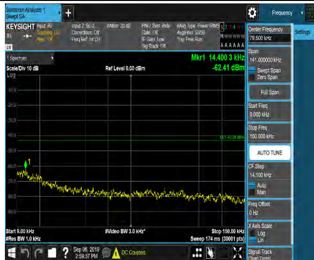
LTE Band 2_1.4MHz_QPSK_19193_1RB#0_Range2:0.15~30MHz_-57.76_PASS
