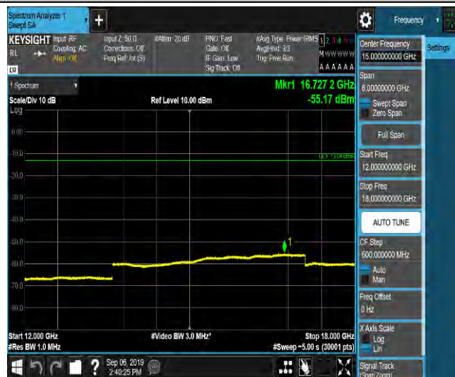
LTE Band 2_1.4MHz_QPSK_19193_1RB#0_Range1:0.009~0.15MHz_-62.41_PASS
