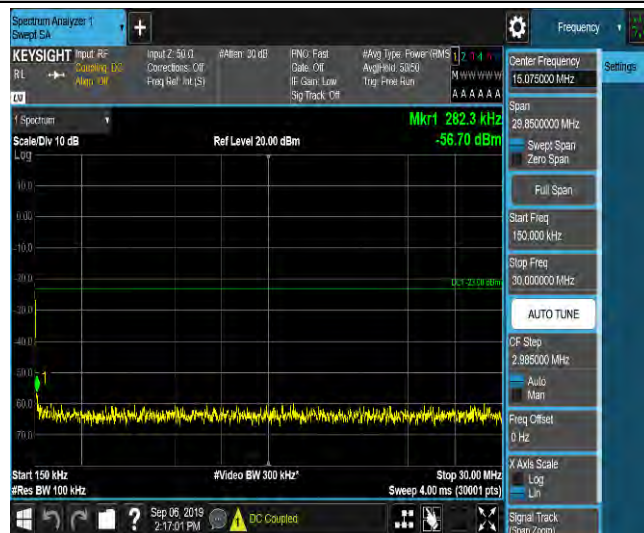
LTE Band 2_1.4MHz_16QAM_18607_1RB#0_Range3:30~1000MHz_-46.58_PASS
