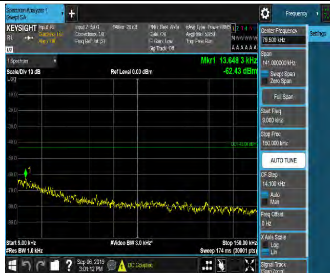
LTE Band 2_1.4MHz_16QAM_19193_1RB#0_Range2:0.15~30MHz_-57.09_PASS
