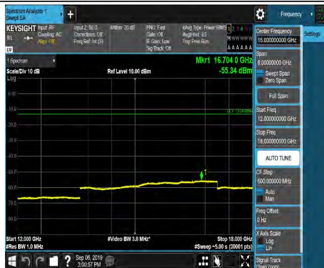
LTE Band 2_1.4MHz_16QAM_19193_1RB#0_Range1:0.009~0.15MHz_-62.43_PASS
