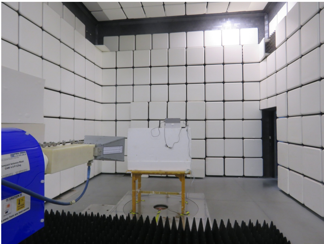
Radiated Spurious Emissions Test setup
