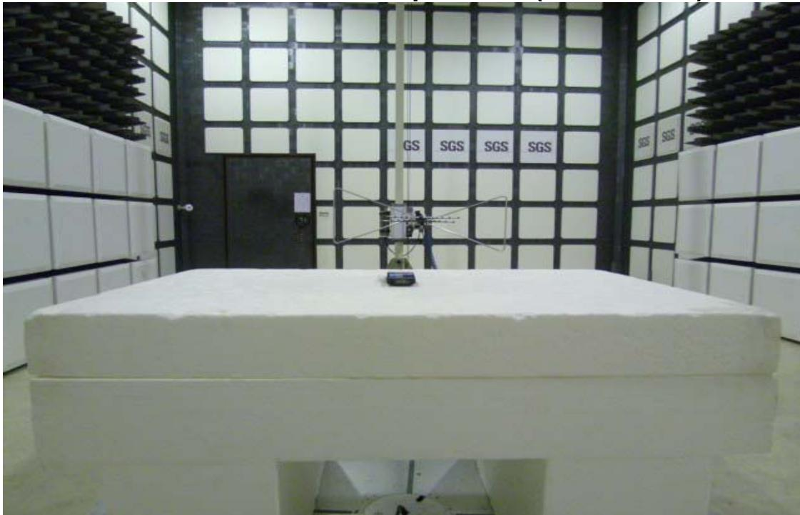
**Radiated Emission Set up Photos (Above 1GHz)**
