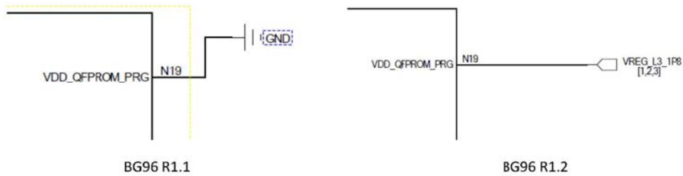
Figure 1: Schematic Designs of BG96 R1.1 and R1.2
