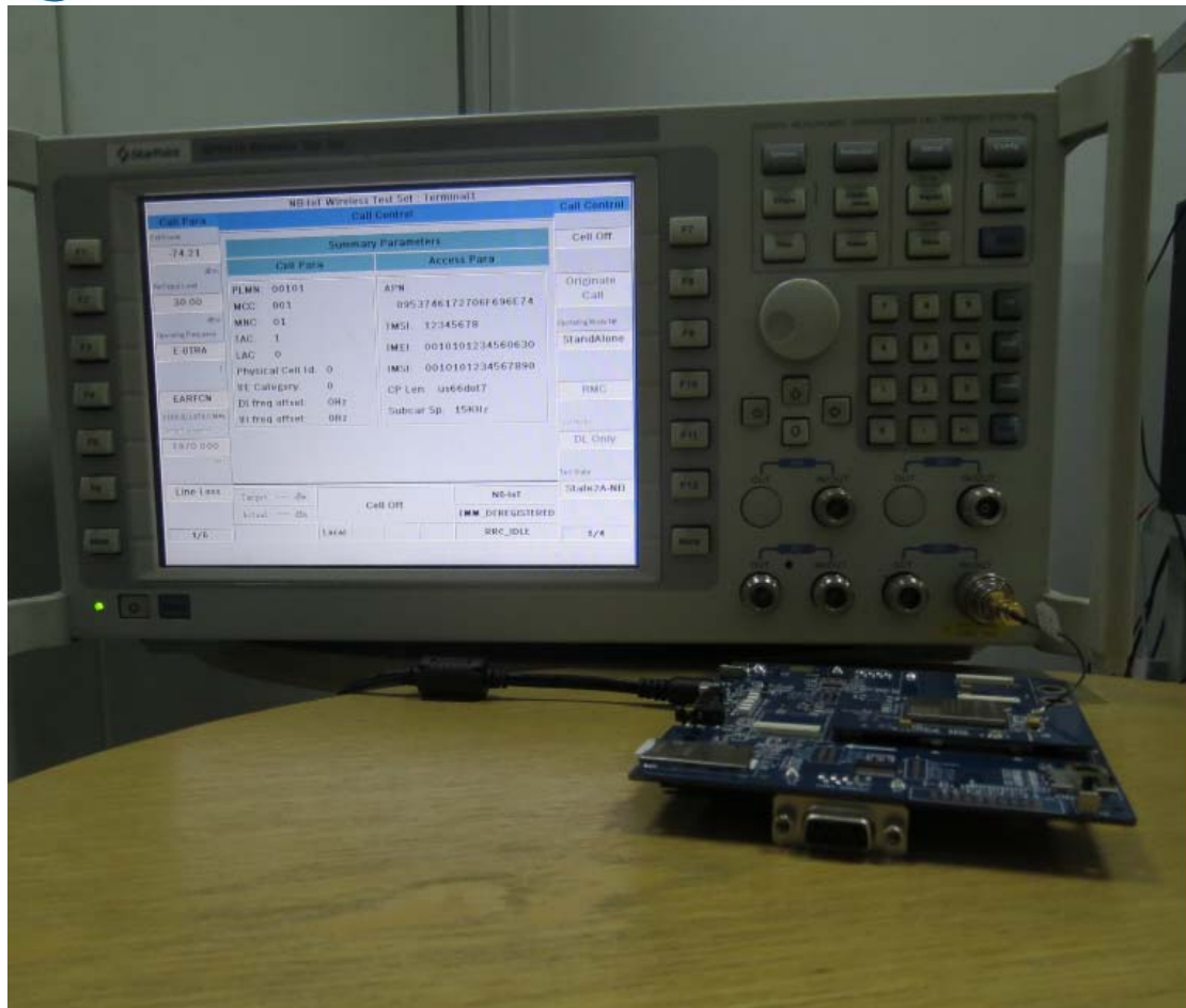
RF conducted test setup
