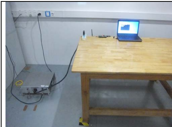
Conducted Emissions Test Setup Front View
