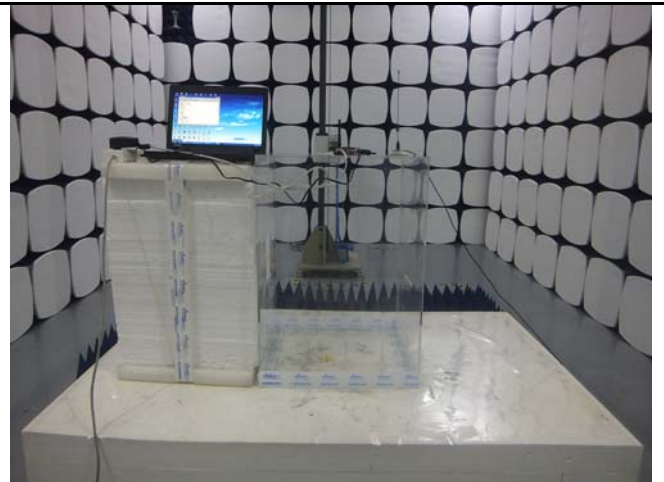
Radiated Spurious Emissions Test Setup Above 1GHz
