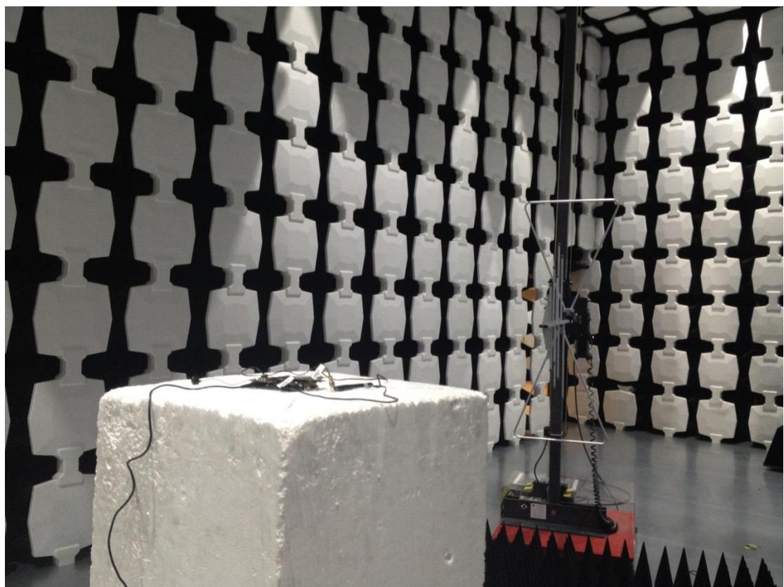
Description: Substitution Antenna for ERP Test
