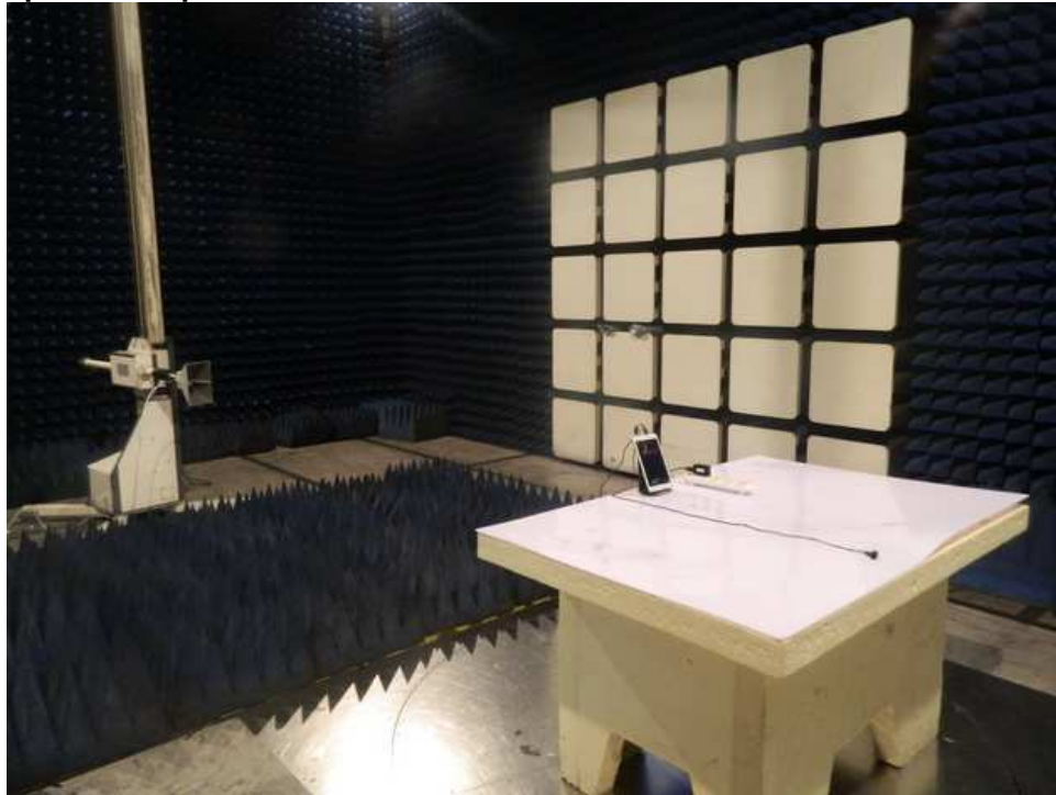
Photograph 3: Set-up for Radiated Emission of 1 - 6GHz
