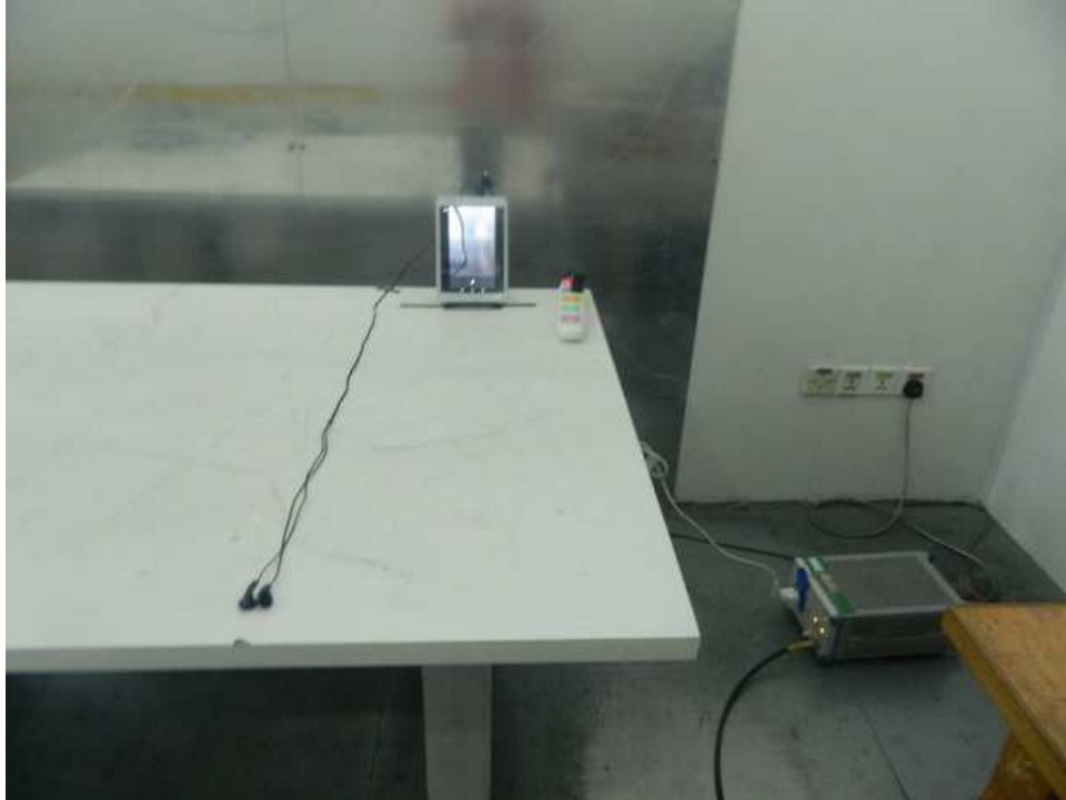
Photograph 1: Set-up for Conducted Emission
