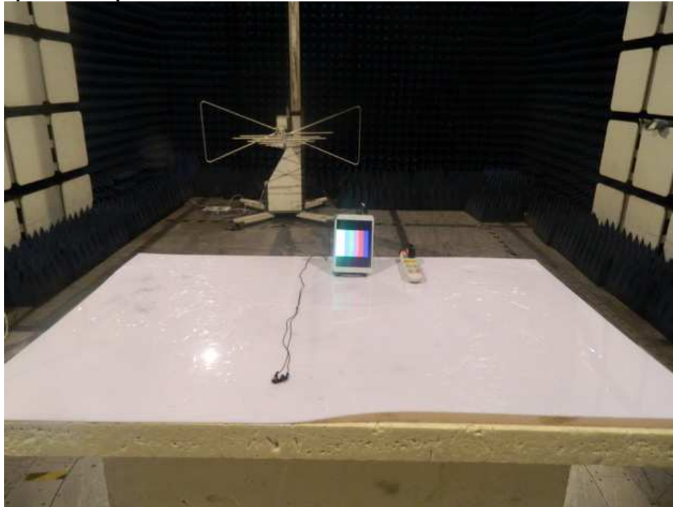
Photograph 2: Set-up for Radiated Emission of below 1GHz
