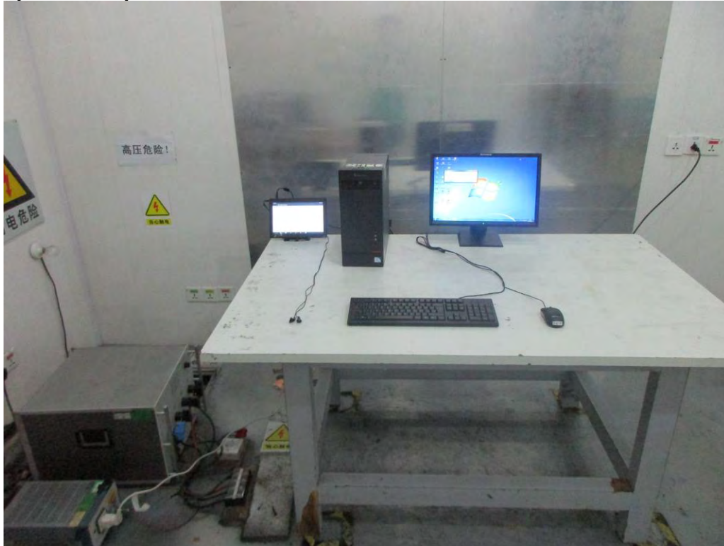
Photograph 2: Set-up for Radiated Emission of below 1GHz
