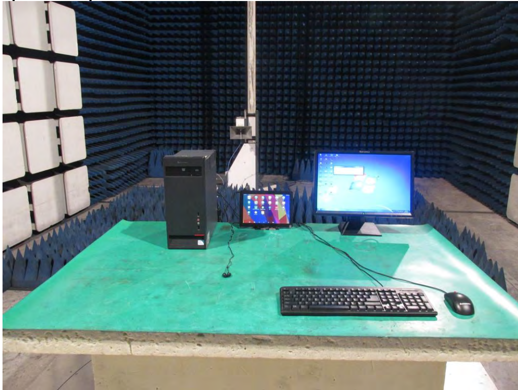
Photograph 3: Set-up for Radiated Emission of 1 - 18GHz
