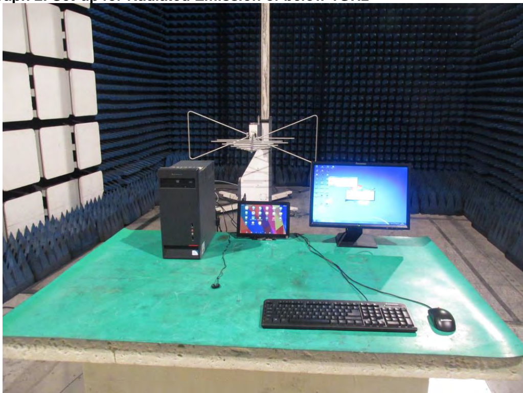
Photograph 2: Set-up for Radiated Emission of below 1GHz
