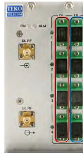
Fiber Optic Module equipped with 1 Transmitter split by 4 and 4 combined Receivers
