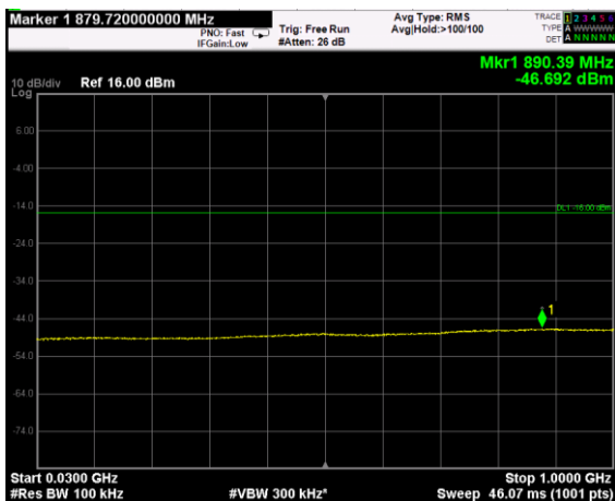
Channel: TOP, Modulation: 64QAM, BW=15MHz, Range: Lower
