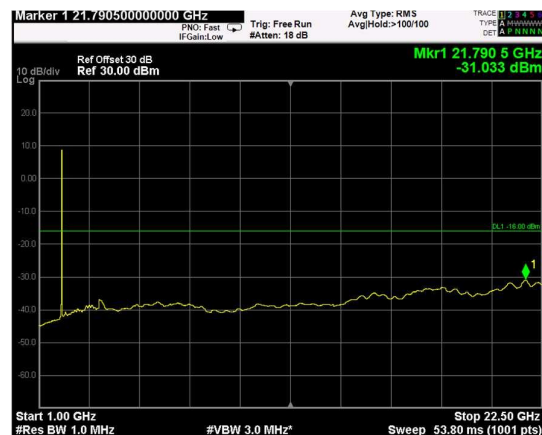
Channel: TOP, Modulation: 16QAM, BW=15MHz, Range: Upper
