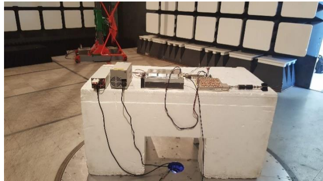
Figure 9.1-2: Radiated setup photo below 1 GHz
