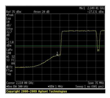
Spurious Emissions at Antenna Terminals Downlink – 15 QPSK HIGH BAND EDGE
