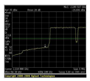
Spurious Emissions at Antenna Terminals Downlink – 3 QAM HIGH BAND EDGE
