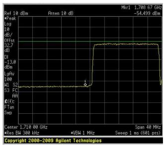
Spurious Emissions at Antenna Terminals Uplink – 20 QPSK HIGH BAND EDGE
