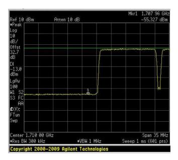
Spurious Emissions at Antenna Terminals Uplink – 15 QAM HIGH BAND EDGE
