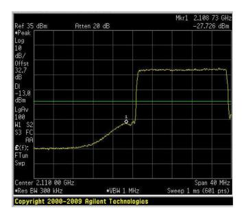
Spurious Emissions at Antenna Terminals Downlink – 20 QPSK HIGH BAND EDGE
