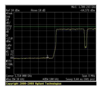
Spurious Emissions at Antenna Terminals Uplink – 3 QAM HIGH BAND EDGE
