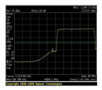
Spurious Emissions at Antenna Terminals Downlink – 20 QAM HIGH BAND EDGE
