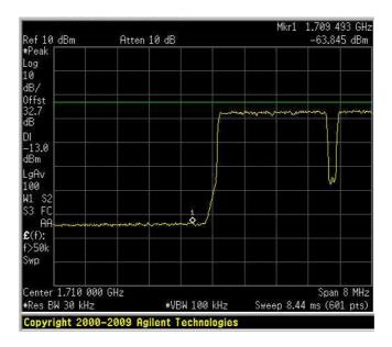
Spurious Emissions at Antenna Terminals Uplink – 3 QPSK HIGH BAND EDGE
