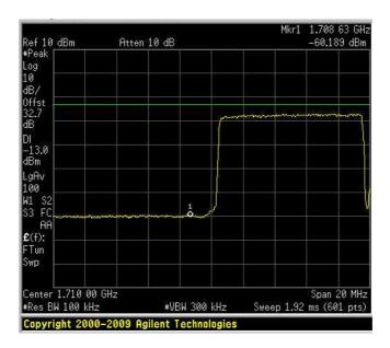
Spurious Emissions at Antenna Terminals Uplink – 10 QAM HIGH BAND EDGE
