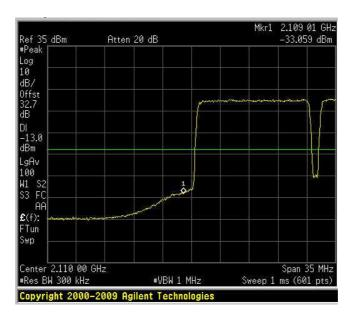
Spurious Emissions at Antenna Terminals Downlink – 15 QAM HIGH BAND EDGE
