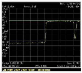
Spurious Emissions at Antenna Terminals Uplink – 15 QPSK HIGH BAND EDGE
