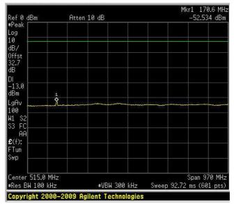
Spurious Emissions at Antenna Terminals Downlink – 10 QPSK 30MHz – 1 GHz
