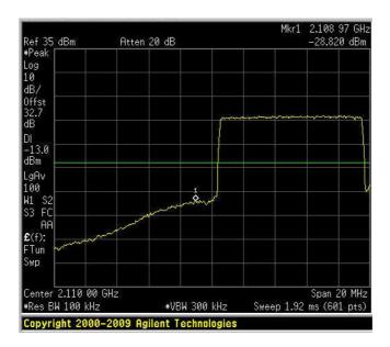
Spurious Emissions at Antenna Terminals Downlink – 10 QPSK HIGH BAND EDGE
