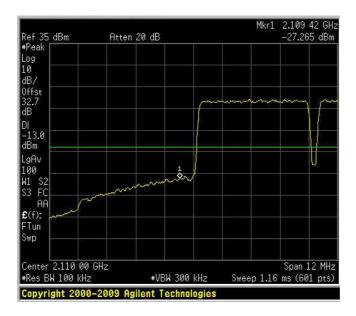
Spurious Emissions at Antenna Terminals Downlink – 5 QAM HIGH BAND EDGE
