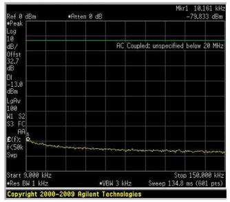
Only 1,4 QAM 9kHz-150kHz spurious emission plots are included here, other modulations spurious emission plots are negligible and the same.
