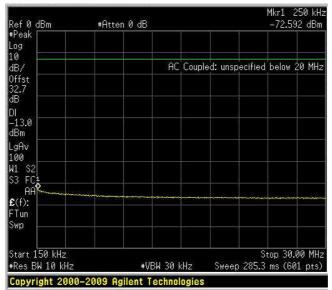
Only 1,4 QAM 150kHz-30MHz spurious emission plots are included here, other modulations spurious emission plots are negligible and the same.
