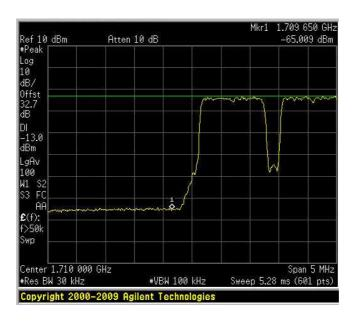
Spurious Emissions at Antenna Terminals Uplink – 1.4 QAM HIGH BAND EDGE
