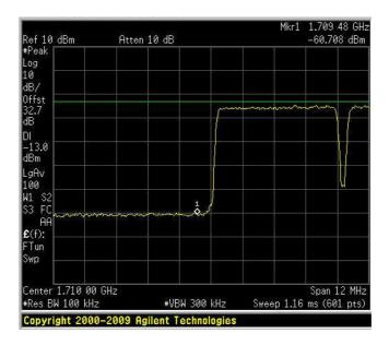
Spurious Emissions at Antenna Terminals Uplink – 5 QAM HIGH BAND EDGE
