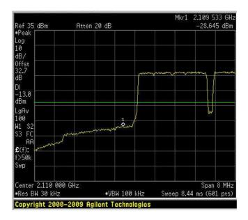
Spurious Emissions at Antenna Terminals Downlink – 3 QPSK HIGH BAND EDGE
