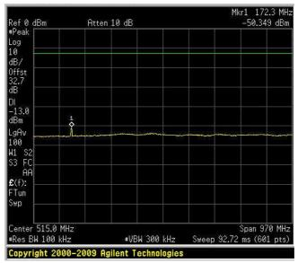
Spurious Emissions at Antenna Terminals Downlink – 5 QPSK 30MHz – 1 GHz
