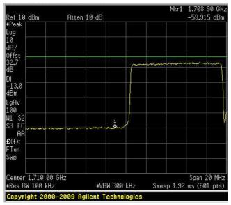
Spurious Emissions at Antenna Terminals Uplink – 10 QPSK HIGH BAND EDGE
