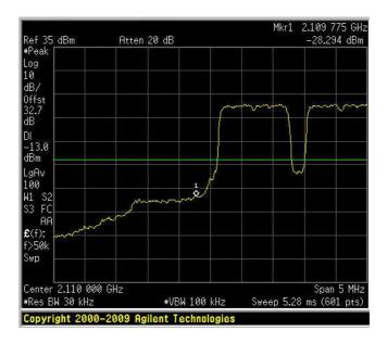
Spurious Emissions at Antenna Terminals Downlink – 1.4 QPSK HIGH BAND EDGE
