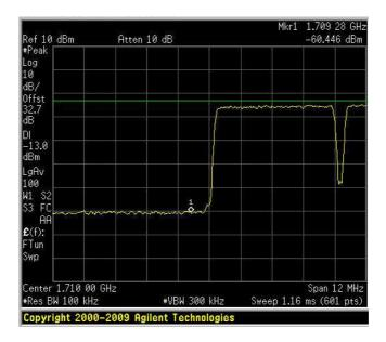
Spurious Emissions at Antenna Terminals Uplink – 5 QPSK HIGH BAND EDGE
