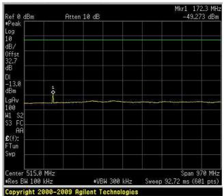
Spurious Emissions at Antenna Terminals Downlink – 3 QPSK 30MHz – 1 GHz
