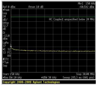
Spurious Emissions at Antenna Terminals Uplink – 1,4 QAM 150 kHz – 30MHz
