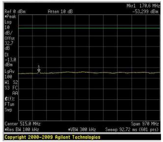
Spurious Emissions at Antenna Terminals Downlink – 20 QPSK 30MHz – 1 GHz
