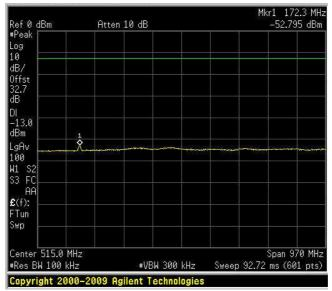
Spurious Emissions at Antenna Terminals Downlink – 15 QPSK 30MHz – 1 GHz
