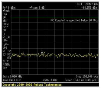
Spurious Emissions at Antenna Terminals Uplink – 1,4 QAM 9 kHz – 150 kHz
