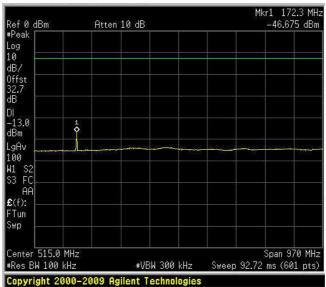
Spurious Emissions at Antenna Terminals Downlink – 1,4 QPSK 30MHz – 1 GHz
