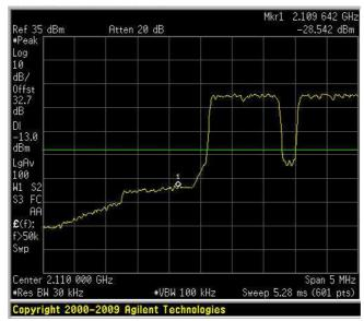
Spurious Emissions at Antenna Terminals Downlink – 1.4 QAM HIGH BAND EDGE
