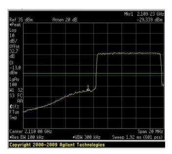
Spurious Emissions at Antenna Terminals Downlink – 10 QAM HIGH BAND EDGE
