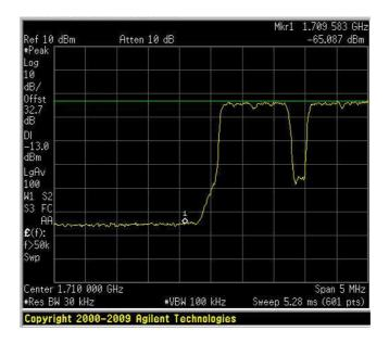
Spurious Emissions at Antenna Terminals Uplink – 1.4 QPSK HIGH BAND EDGE
