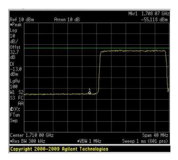
Spurious Emissions at Antenna Terminals Uplink – 20 QAM HIGH BAND EDGE
