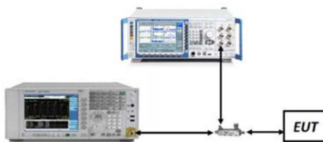
Figure 7-6. ERP/EIRP Measurement Setup
