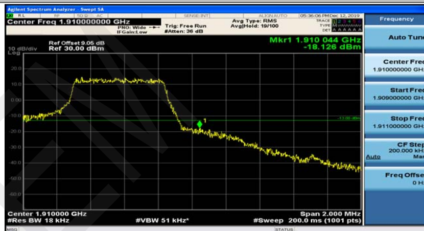
(Channel Bandwidth: 1.4 MHz)_HCH_16QAM_6RB#0
