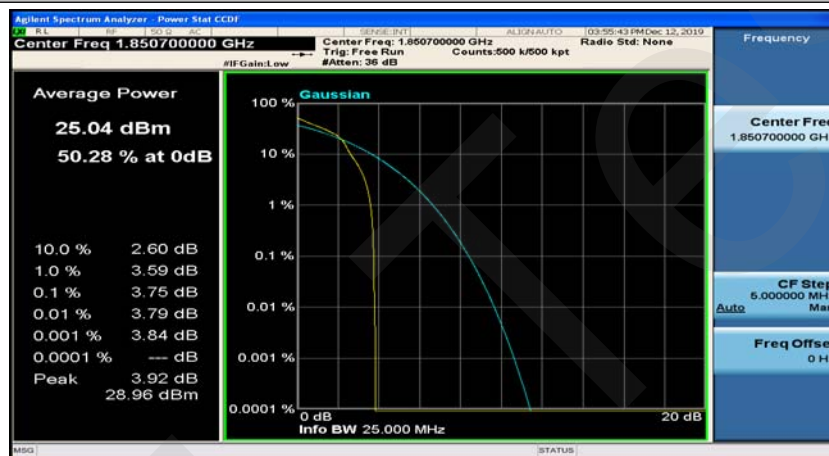
(Channel Bandwidth: 1.4 MHz)_LCH_16QAM_1RB#5
