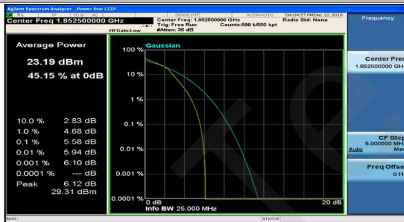
(Channel Bandwidth: 5 MHz)_LCH_16QAM_12RB#13
