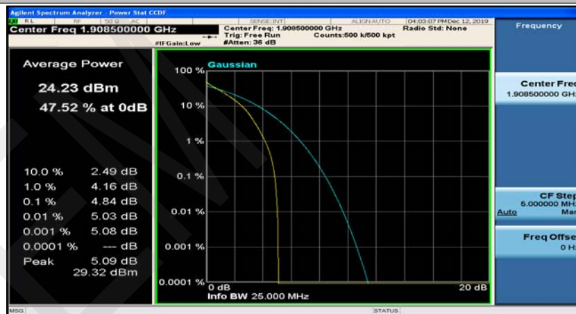
(Channel Bandwidth: 3 MHz)_HCH_QPSK_8RB#4
