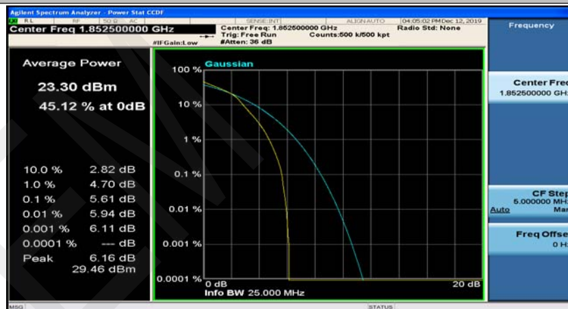
(Channel Bandwidth: 5 MHz)_LCH_16QAM_25RB#0
