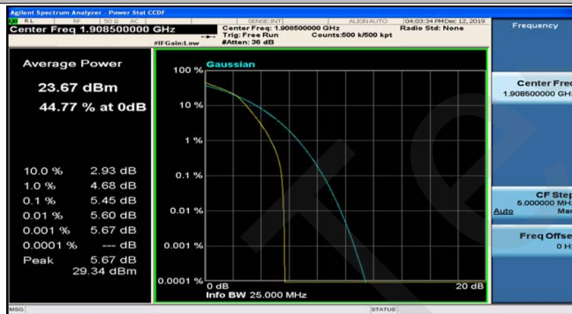
(Channel Bandwidth: 3 MHz)_HCH_16QAM_15RB#0
