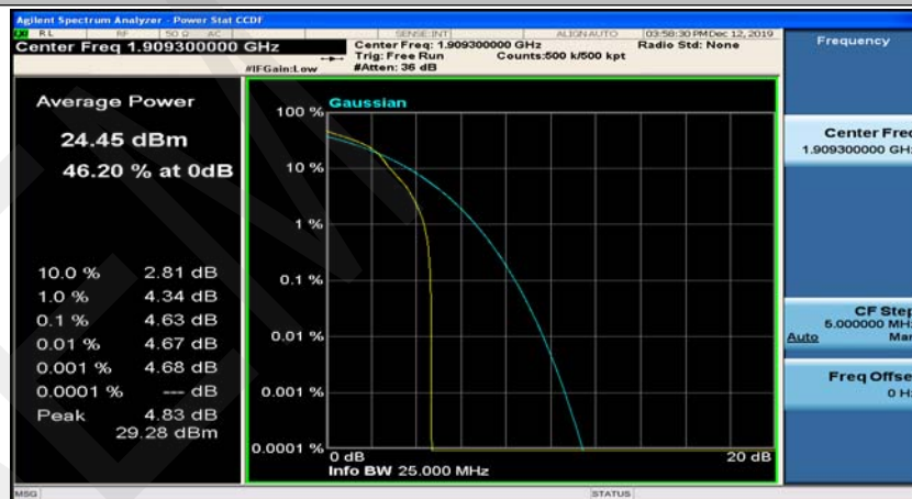
(Channel Bandwidth: 1.4 MHz)_HCH_16QAM_1RB#3
