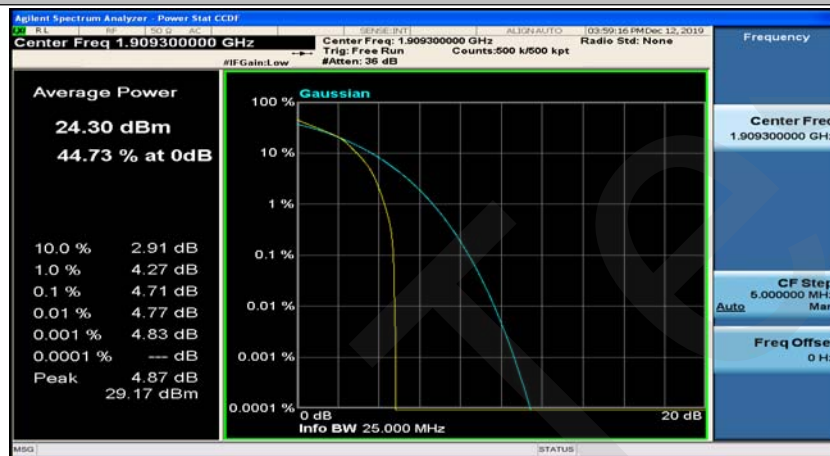
(Channel Bandwidth: 1.4 MHz)_HCH_16QAM_6RB#0
