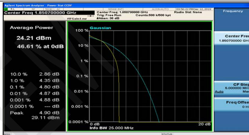
(Channel Bandwidth: 1.4 MHz)_LCH_16QAM_6RB#0
