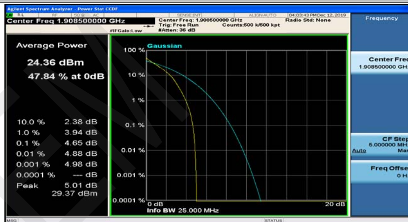
(Channel Bandwidth: 3 MHz)_HCH_QPSK_15RB#0
