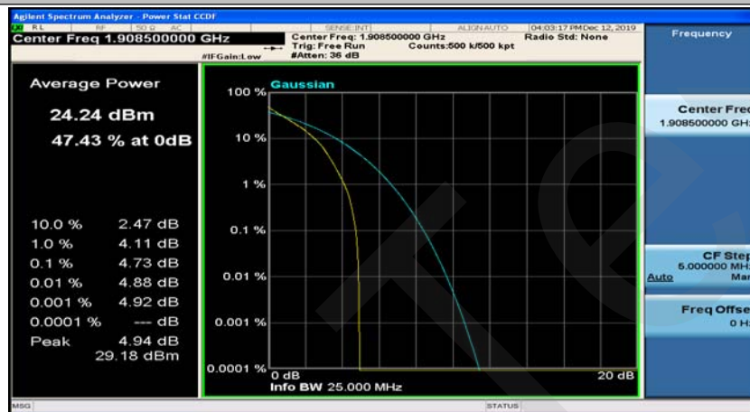
(Channel Bandwidth: 3 MHz)_HCH_QPSK_15RB#0
