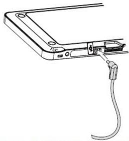
To charge the battery, pry open the rubber cover protecting the DC-in port and plug in the AC adaptor cable supplied with the tablet.
