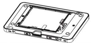
Pry open the battery cover first, and then remove the rubber cover securing the docking board.
