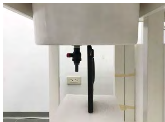
Fig.5 EUT Top side to flat phantom
