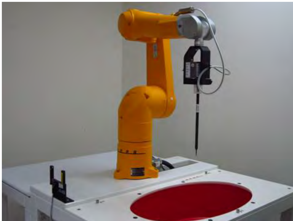
Fig.1 Photograph of the SAR measurement system
