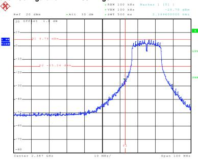
High Band Edge Plot on Configuration IEEE 802.11g / 2462 MHz
