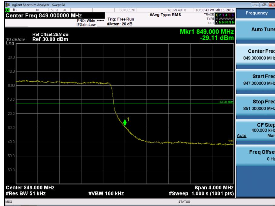
BAND 5. Upper Extended Band Edge Plot (5M BW Ch.20625 QPSK\_RB25\_0)
