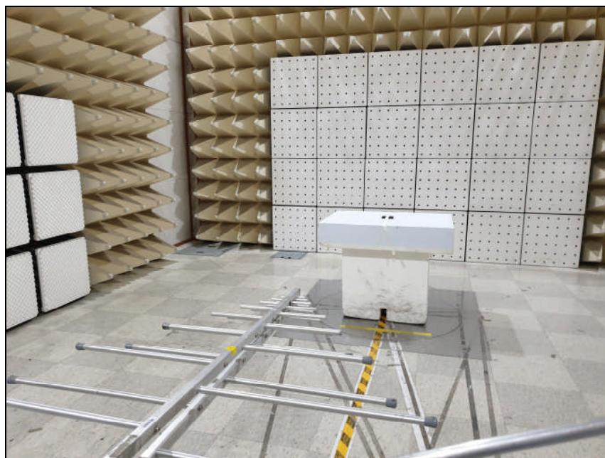
**3. Photo of Radiated Spurious Emission Test (Above 1 GHz)**
