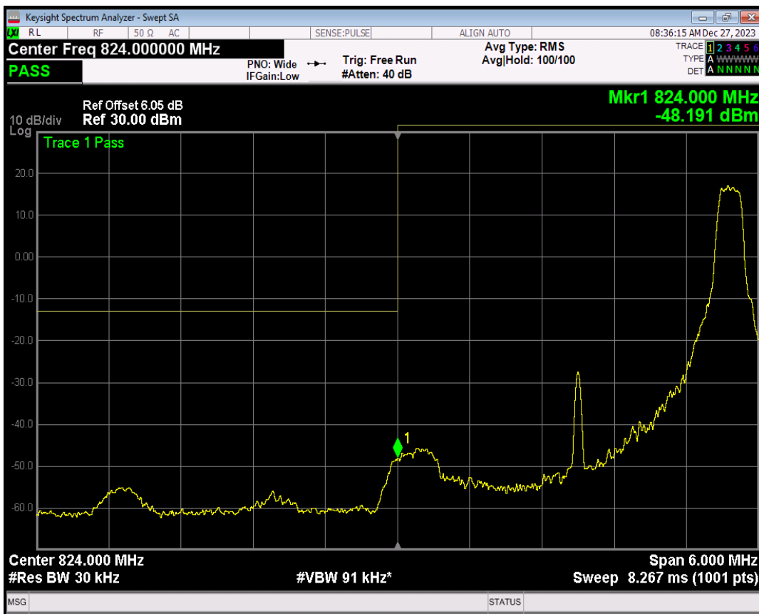
Band26(824-849) QPSK BW=3MHz Channel=26805 RB Size=15 Position=#0
