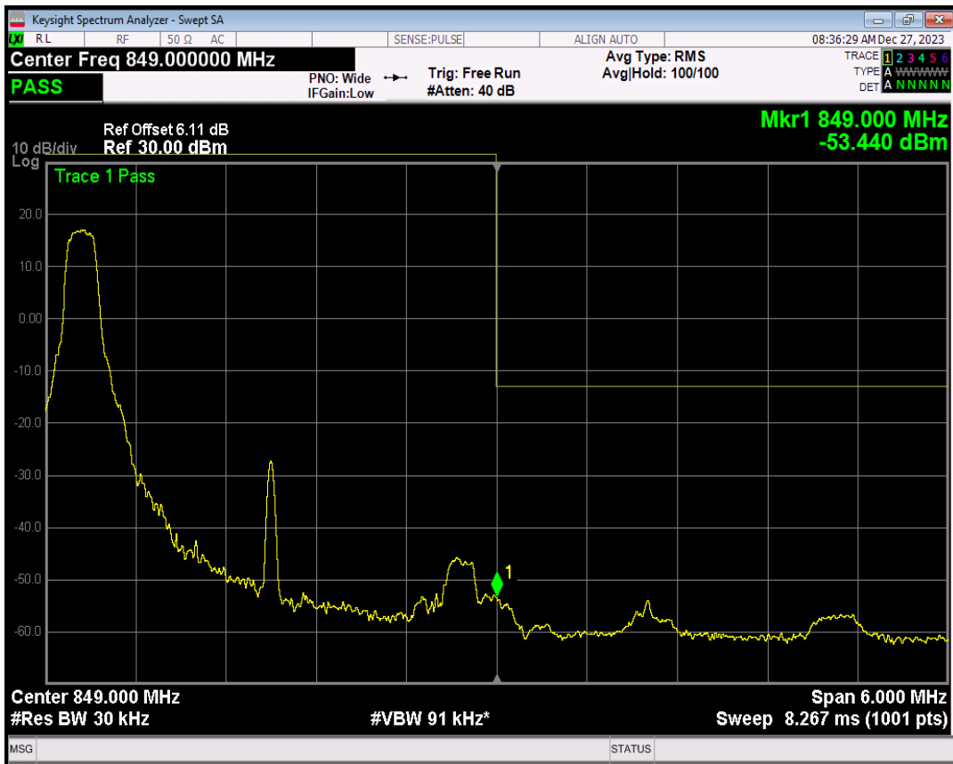
Band26(824-849) QPSK BW=3MHz Channel=27025 RB Size=1 Position=#Max
