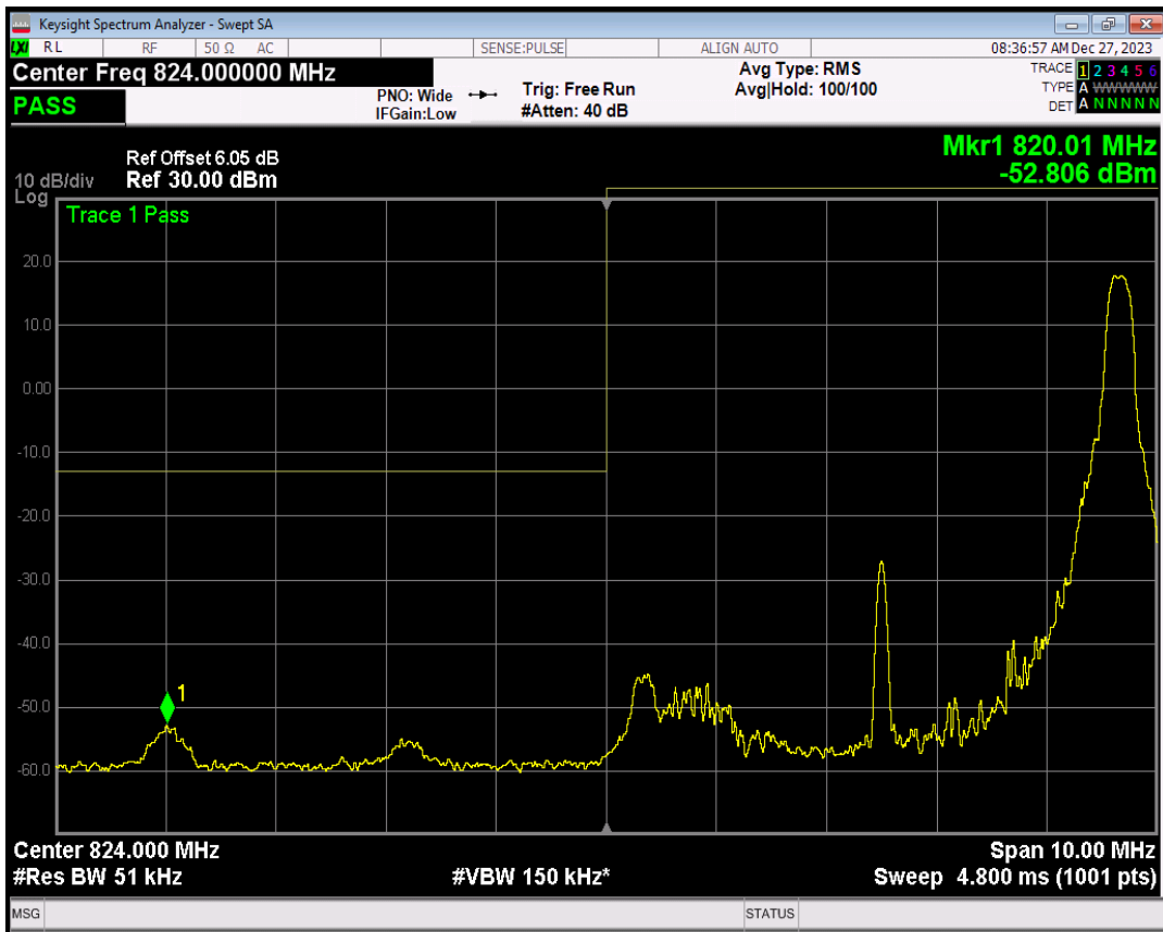
Band26(824-849) 16QAM BW=5MHz Channel=26815 RB Size=25 Position=#0
