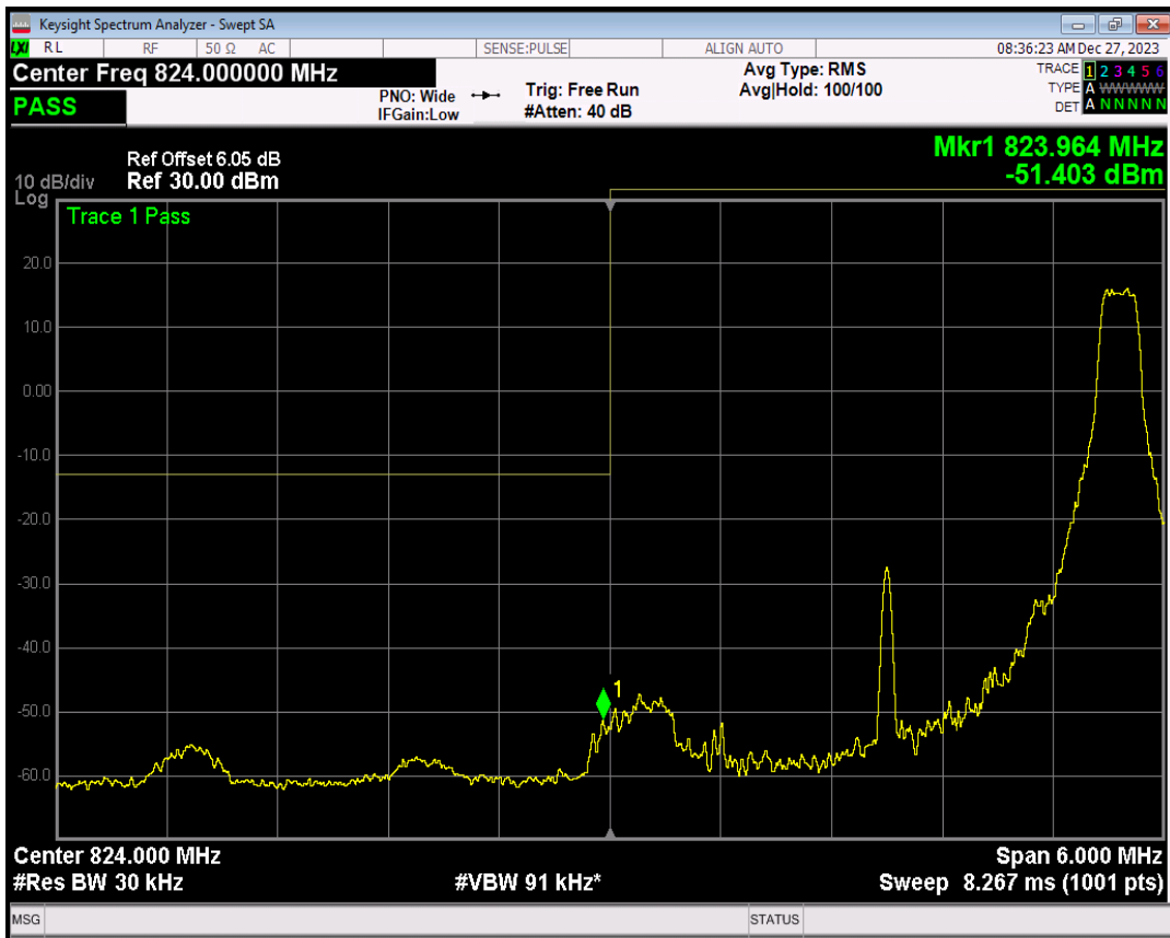
Band26(824-849) 16QAM BW=3MHz Channel=26805 RB Size=15 Position=#0
