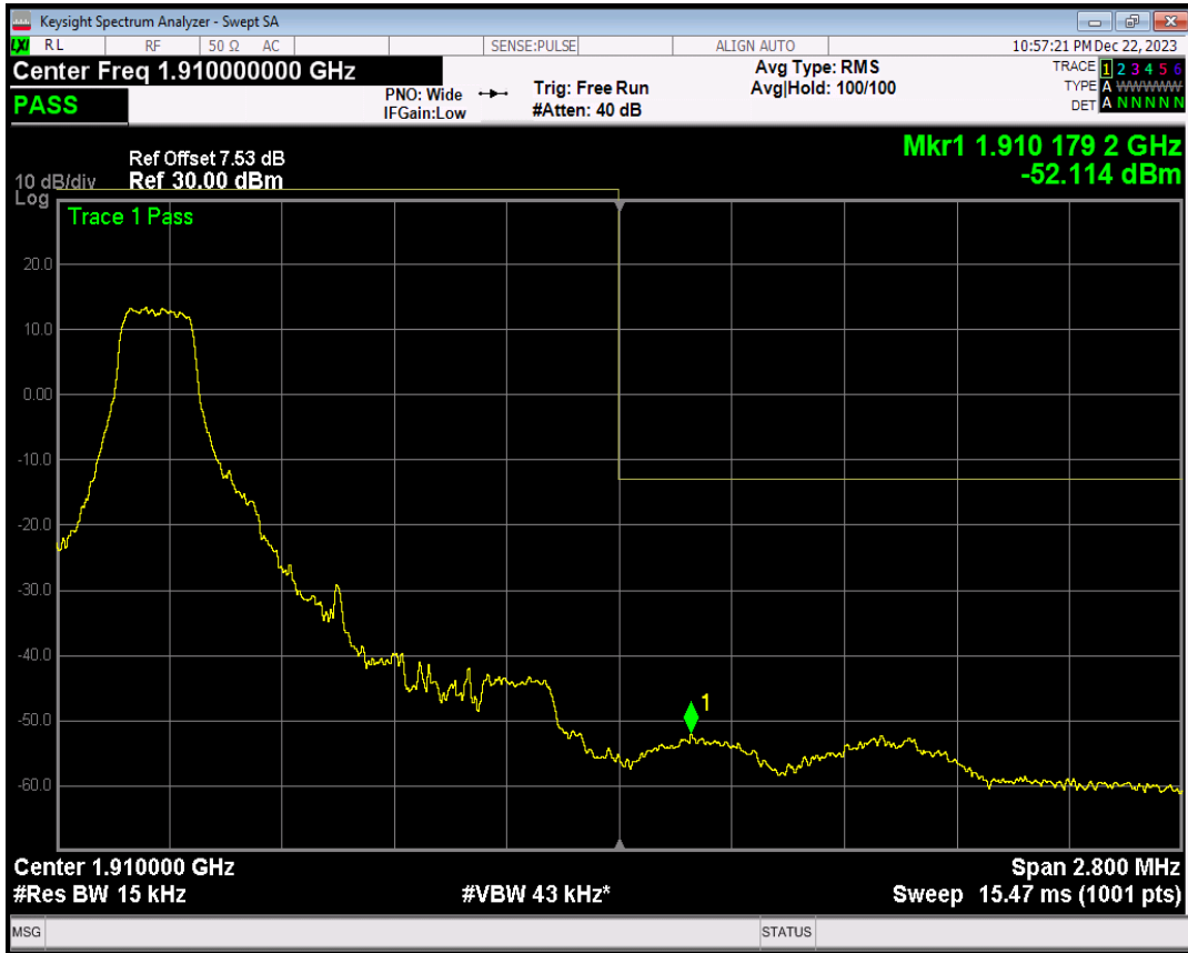
Band2 16QAM BW=1.4MHz Channel=19193 RB Size=1 Position=#Max
