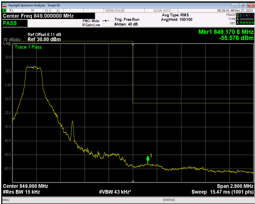
Band26(824-849) QPSK BW=1.4MHz Channel=27033 RB Size=6 Position=#0
