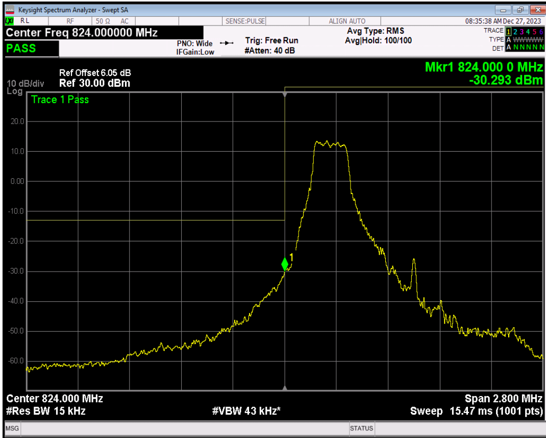
Band26(824-849) 16QAM BW=1.4MHz Channel=26797 RB Size=1 Position=#Max
