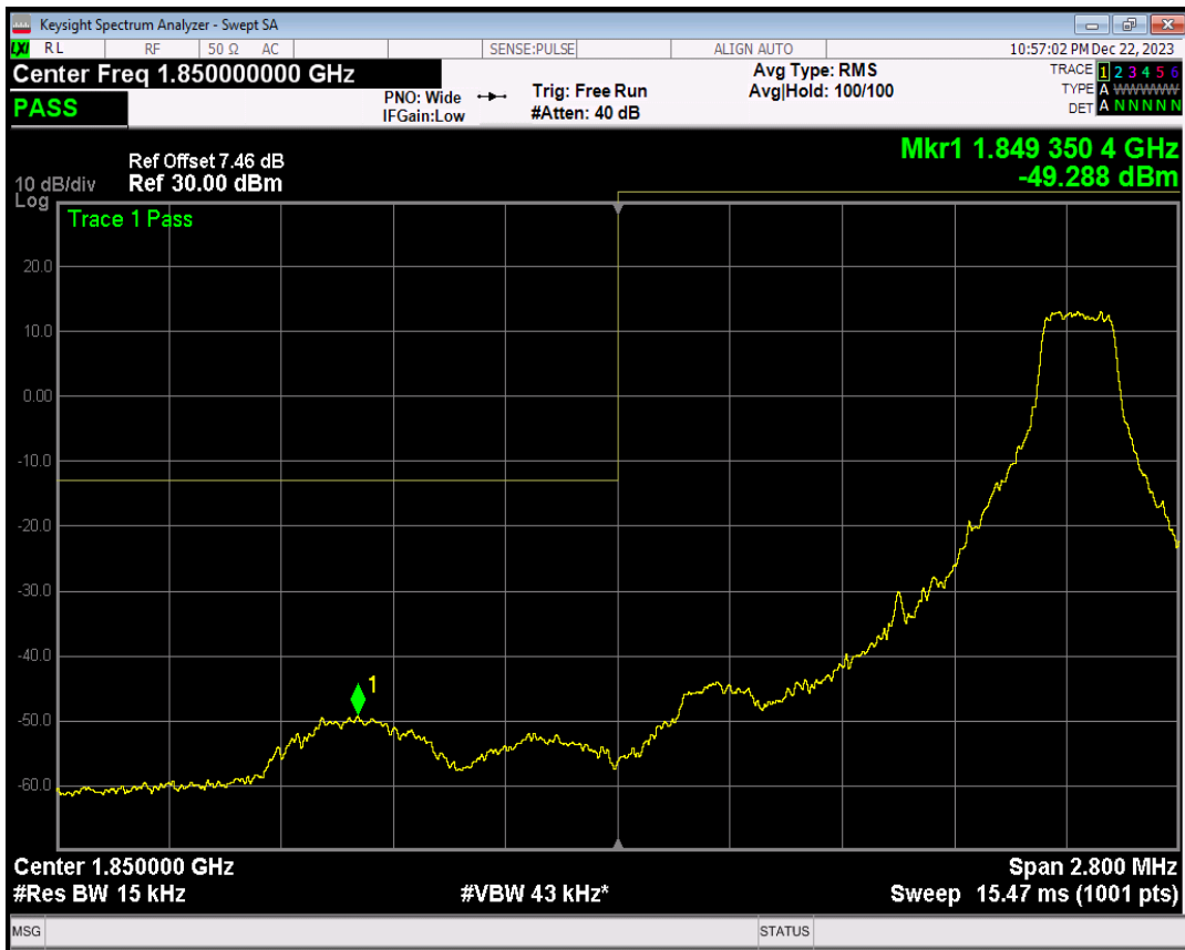
Band2 16QAM BW=1.4MHz Channel=18607 RB Size=6 Position=#0
