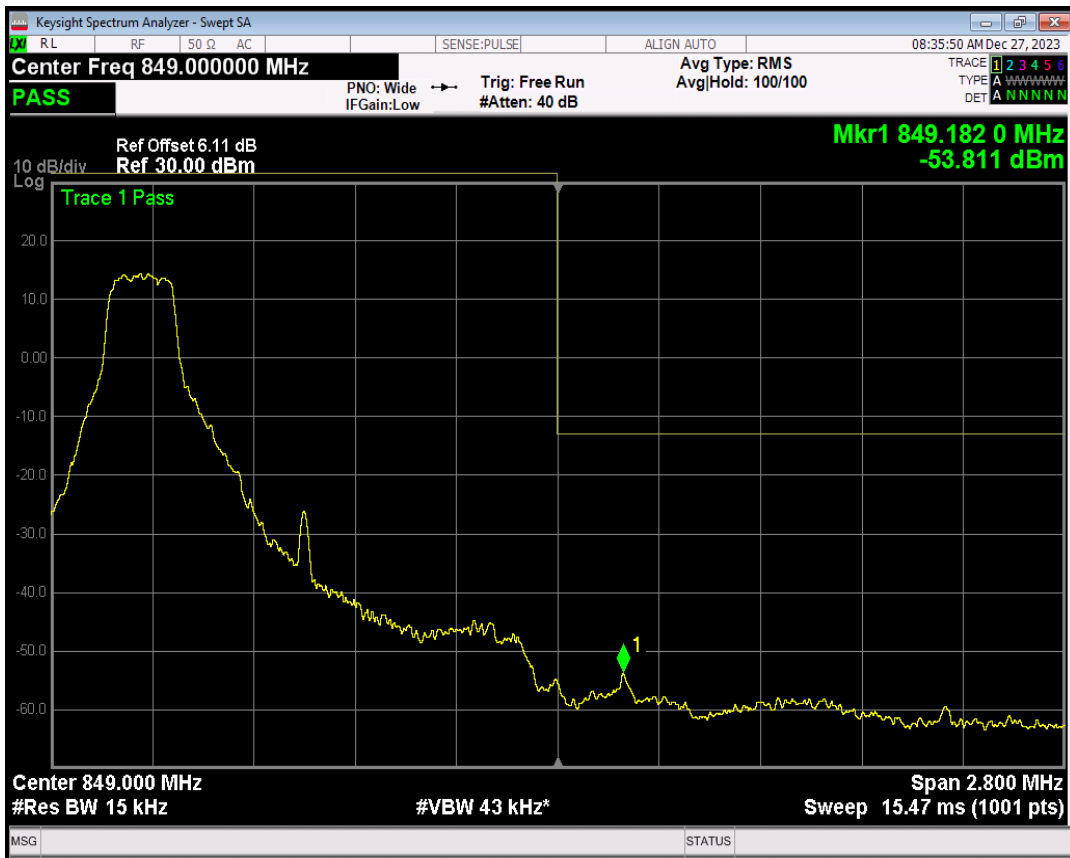
Band26(824-849) QPSK BW=1.4MHz Channel=27033 RB Size=1 Position=#Max
