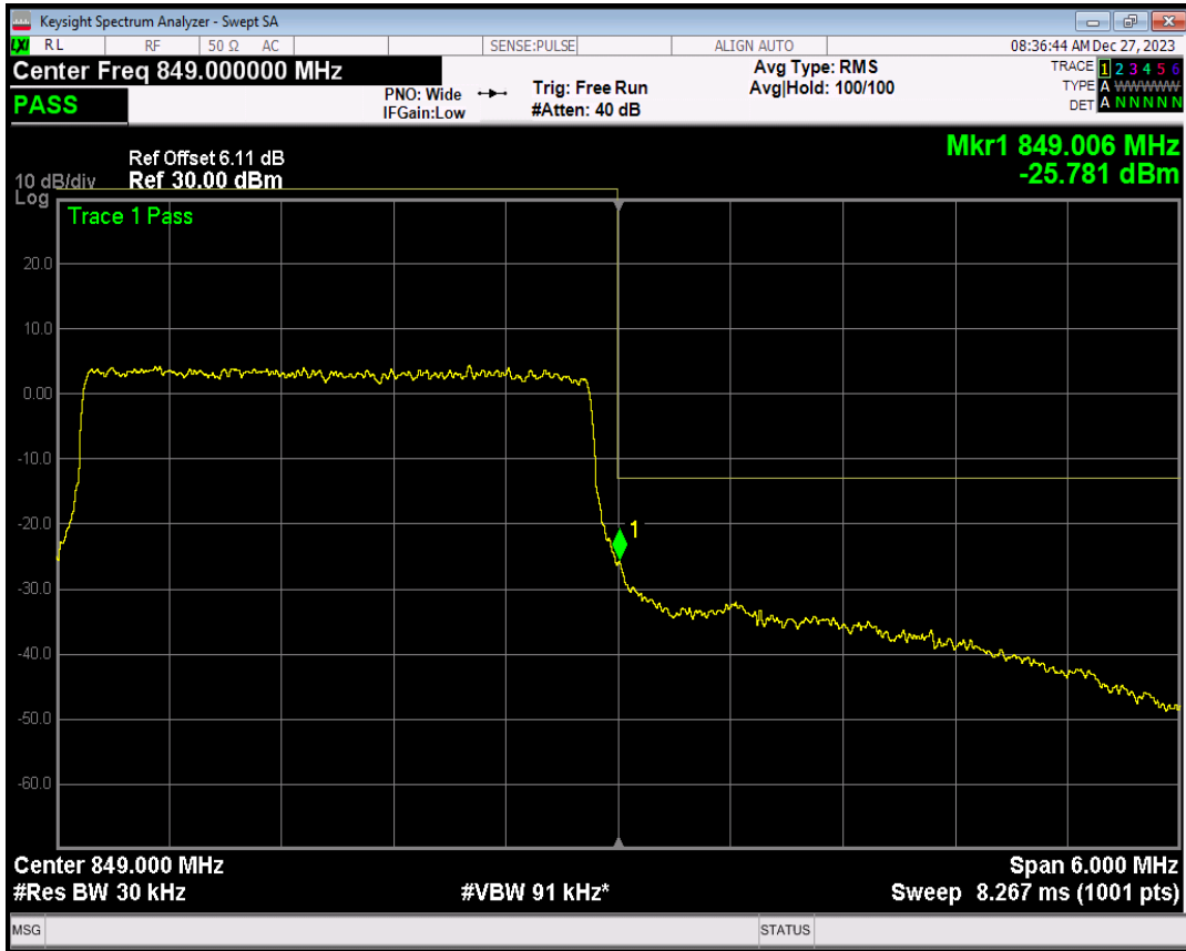
Band26(824-849) QPSK BW=5MHz Channel=26815 RB Size=1 Position=#0
