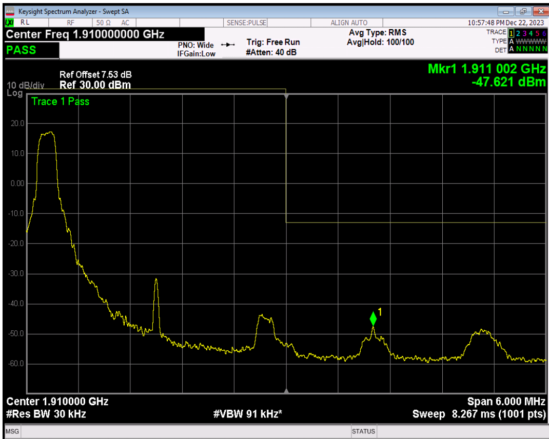
Band2 QPSK BW=3MHz Channel=19185 RB Size=1 Position=#Max
