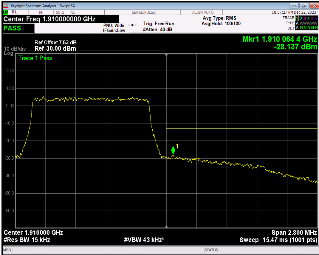
Band2 QPSK BW=3MHz Channel=18615 RB Size=1 Position=#0
