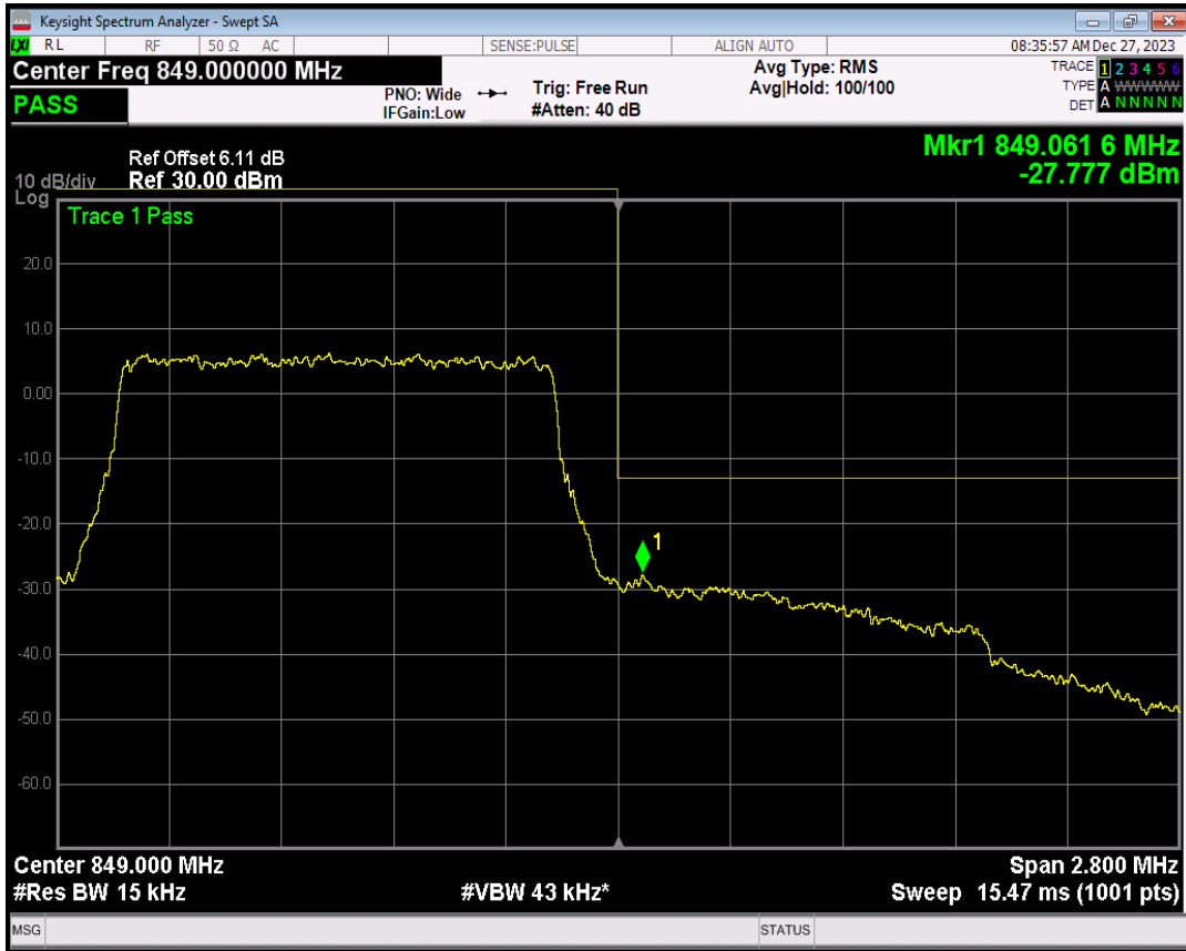
Band26(824-849) 16QAM BW=1.4MHz Channel=27033 RB Size=1 Position=#Max
