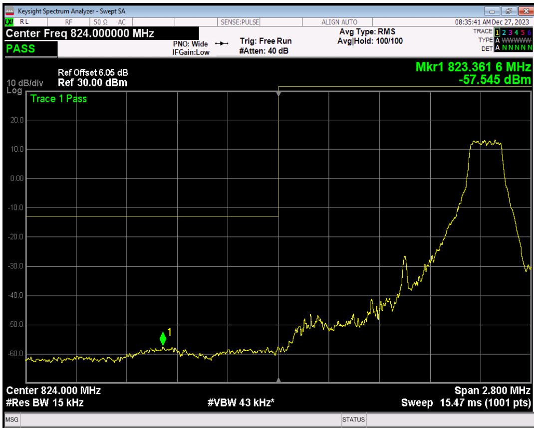
Band26(824-849) 16QAM BW=1.4MHz Channel=26797 RB Size=6 Position=#0
