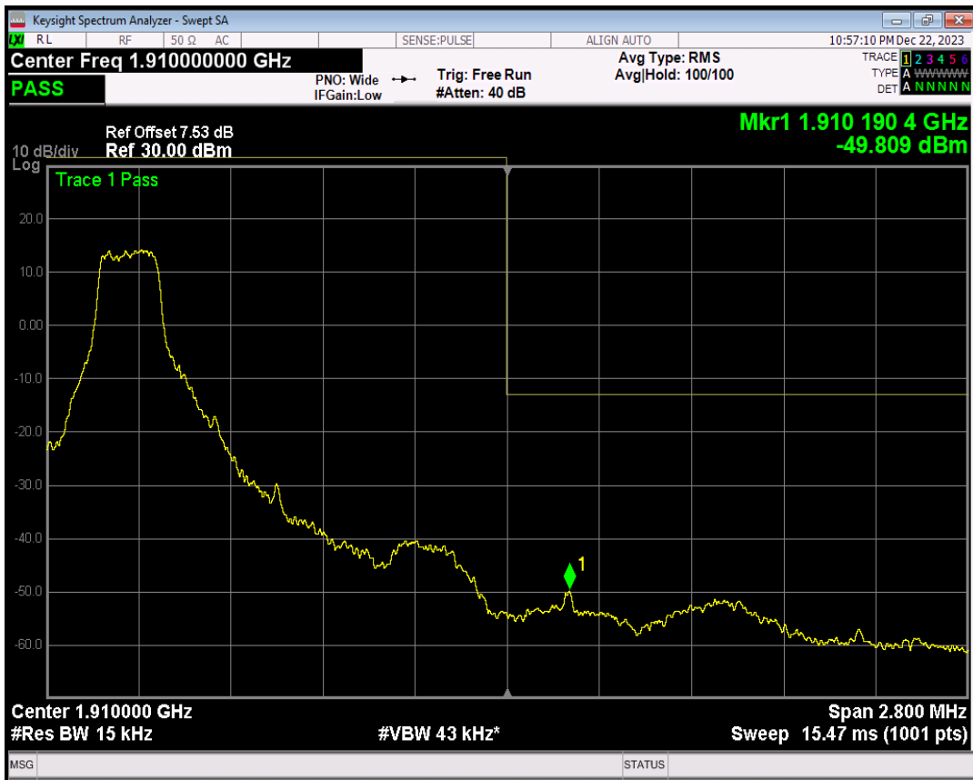
Band2 QPSK BW=1.4MHz Channel=19193 RB Size=1 Position=#Max
