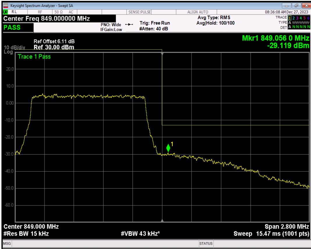
Band26(824-849) QPSK BW=3MHz Channel=26805 RB Size=1 Position=#0
