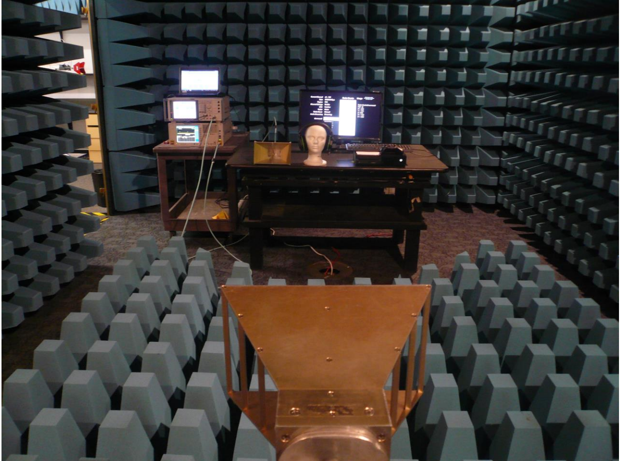
Figure 11: DFS Test Setup (Rear View)
