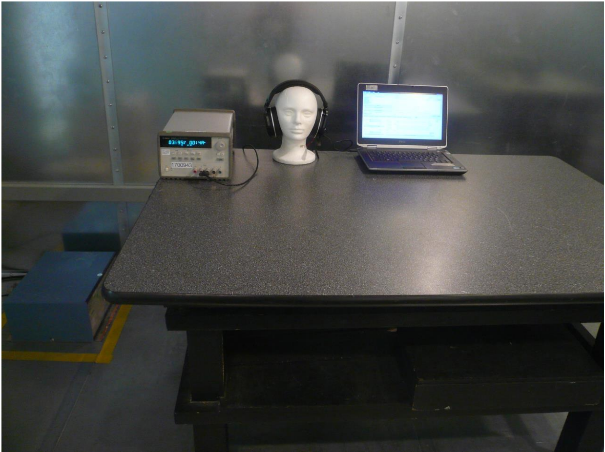
Figure 9: AC Conducted Emission Test Setup (Front)
