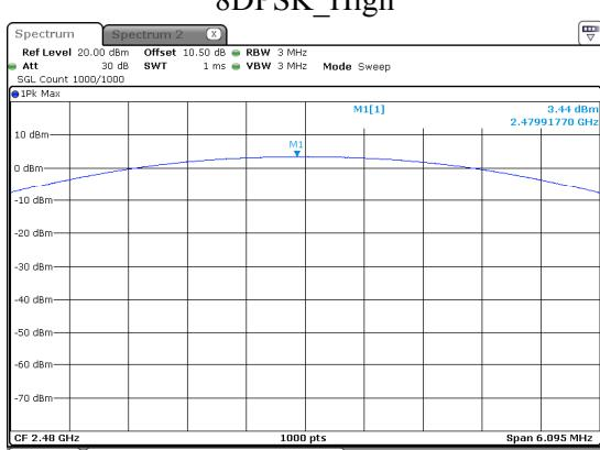
**5.8 100 kHz Bandwidth of Frequency Band Edge**
