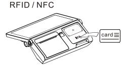
Support ISO14443 TYPE A standard, Mifare standard card, the module integrates instructions such as automatic card searching, reading, writing, initializing e-wallet, adding value, reducing value, checking balance, etc. The recommended swiping distance is 0 to 2 cm.
