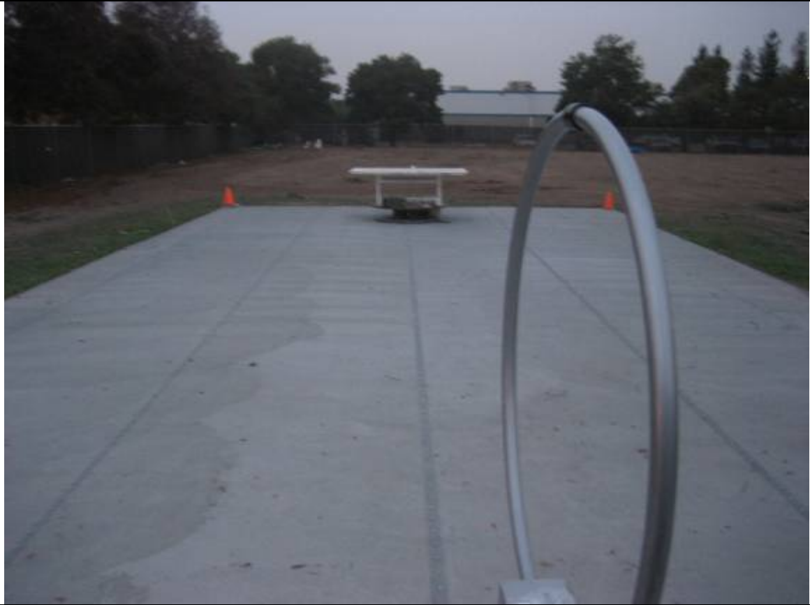
Radiated Emission Test Setup – Front View (<30MHz)
