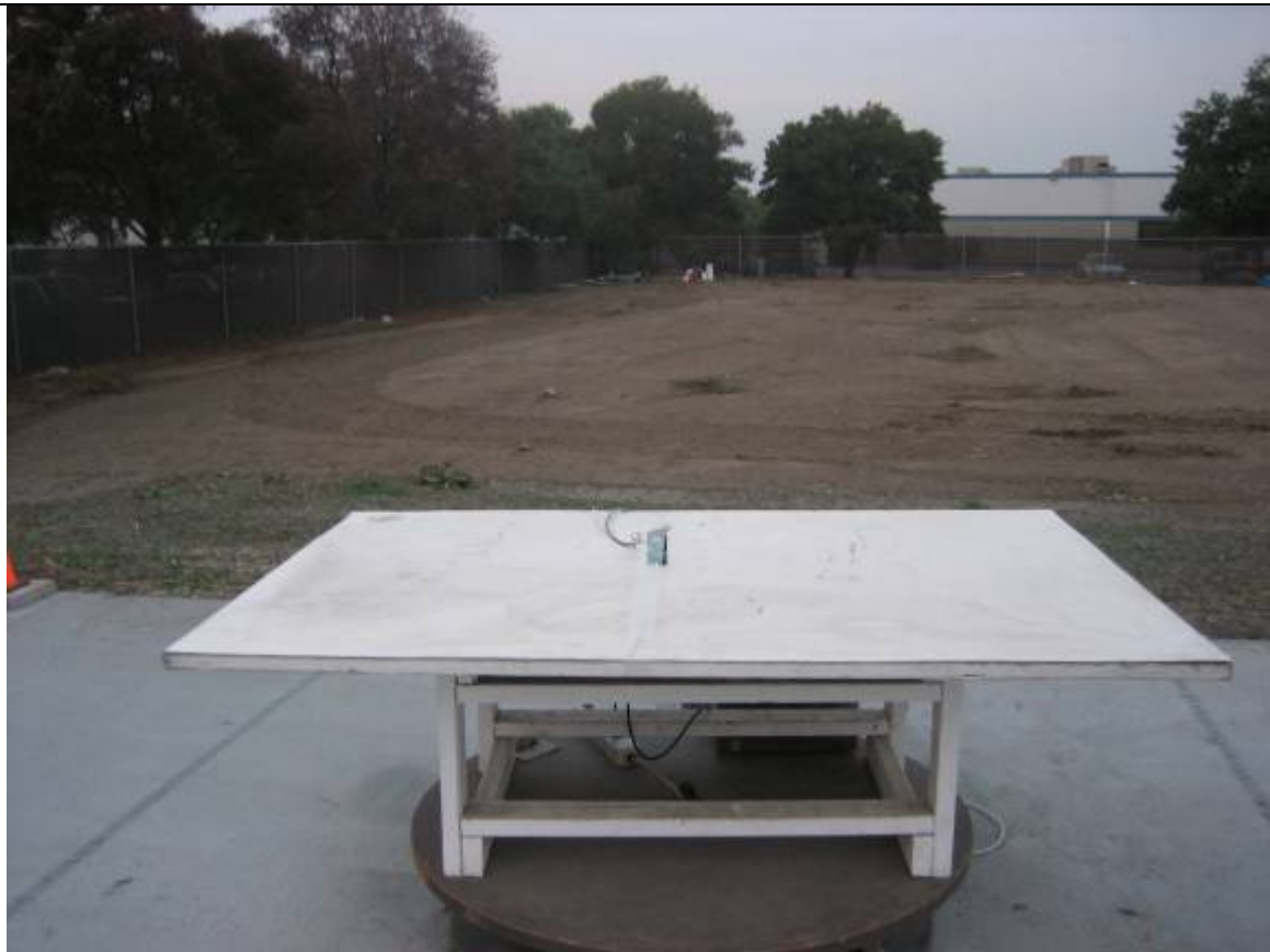
Radiated Emission Test Setup – Front View (>30MHz)
