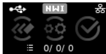
In case of Ethernet connection, the WebGUI is also loaded, when the device is ready for operation, the OLED display shows the following icon:
