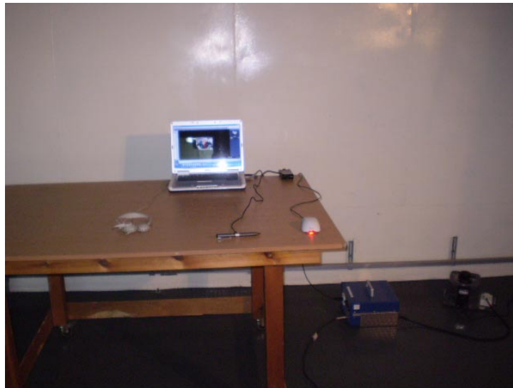
Photograph 7.1.1 Setup for conducted emission measurements
