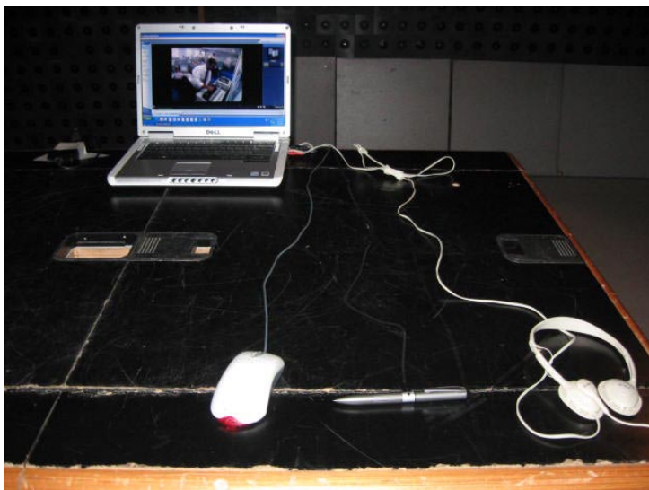
Photograph 7.2.3 Setup for final radiated emission measurements, EUT close view
