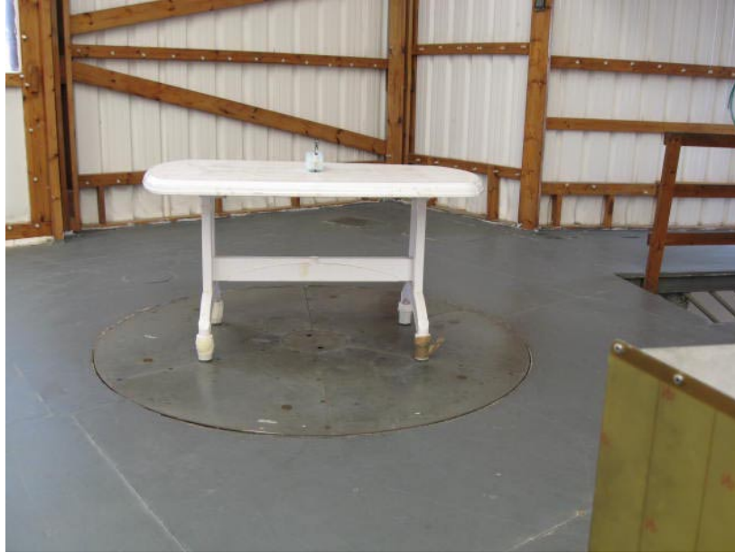
Photograph No.5 Spurious emissions measurement setup above 1000 MHz at the OATS
