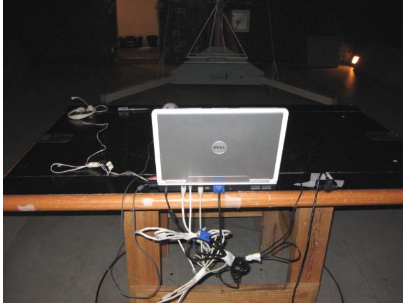
Photograph No.9 Radiated emissions measurement setup in the anechoic chamber, close view
