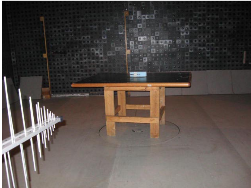
Photograph No.3 Spurious emissions measurement setup in the anechoic chamber in 30-1000 MHz range
