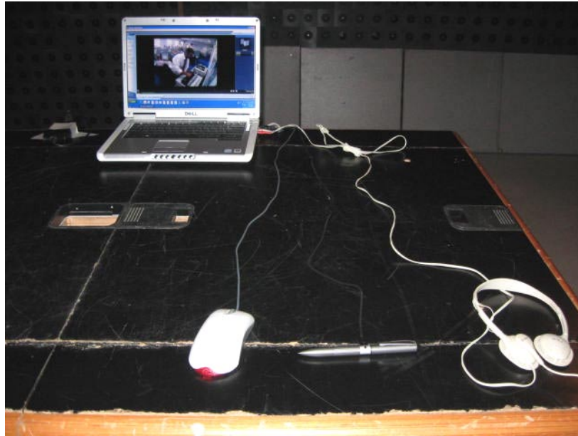
Photograph No.8 Radiated emissions measurement setup in the anechoic chamber, close view
