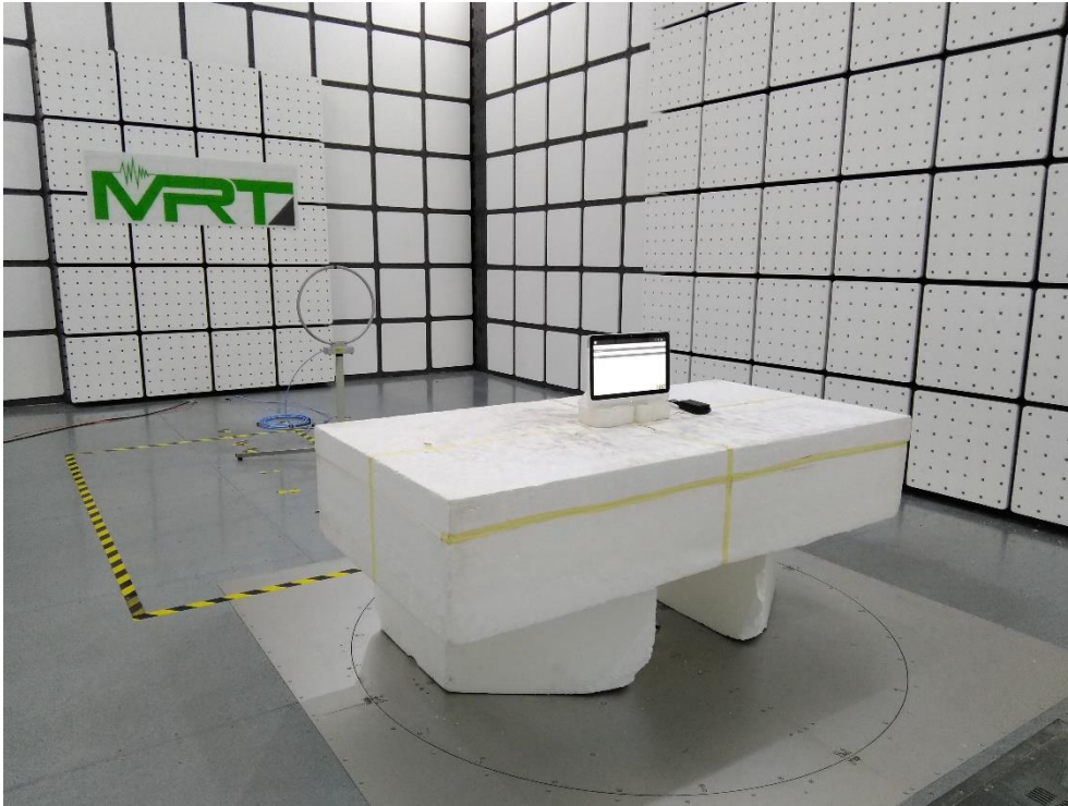
Description: Radiated Emission Test Setup for above 30MHz -Adapter
