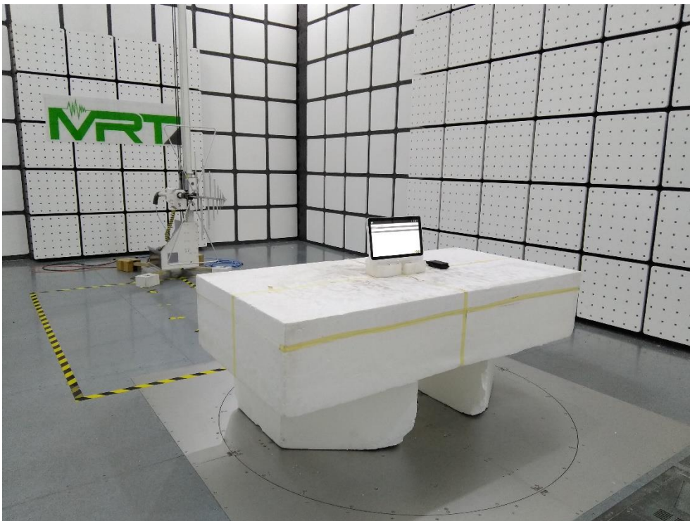
Description: Radiated Emission Test Setup for above 30MHz -Adapter
