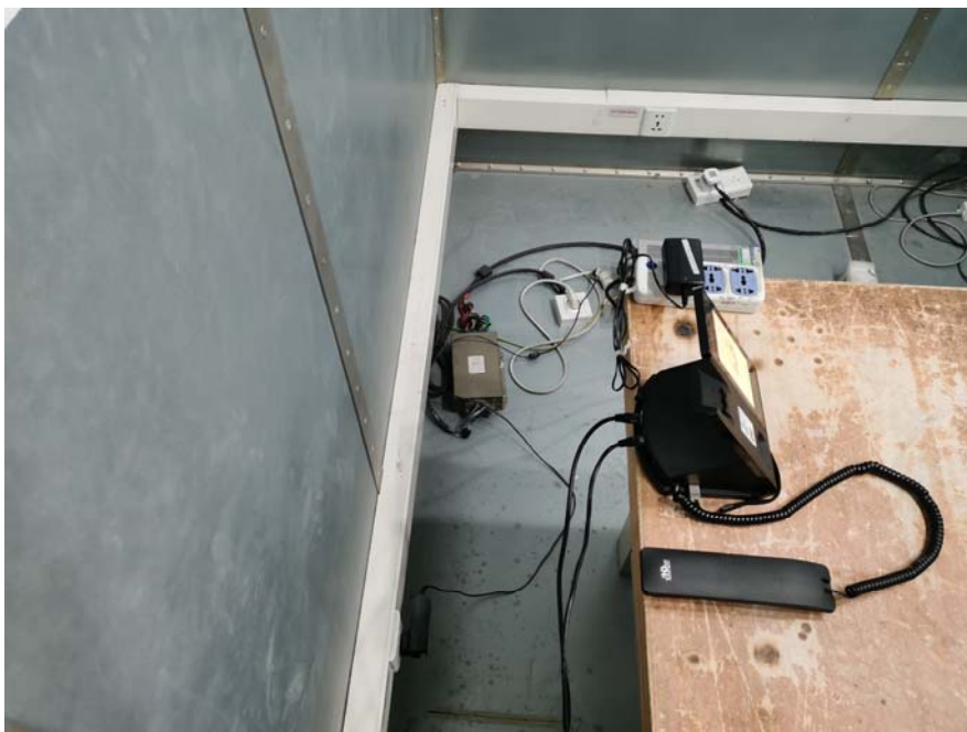
Conducted Emissions - Side View
