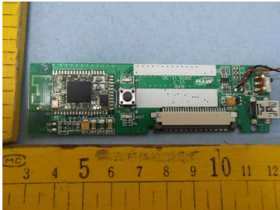
Figure 5 PCB of the EUT-Front View
